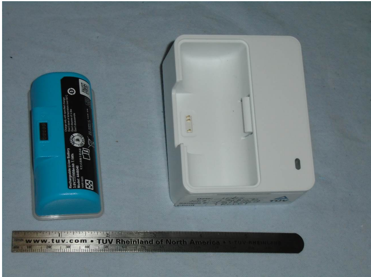
Figure 6: Rear View of battery and charging station.
