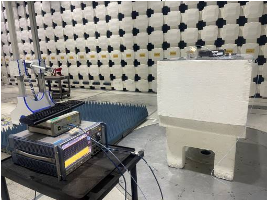
Radiated Emissions Test Setup, 18-26 GHz
