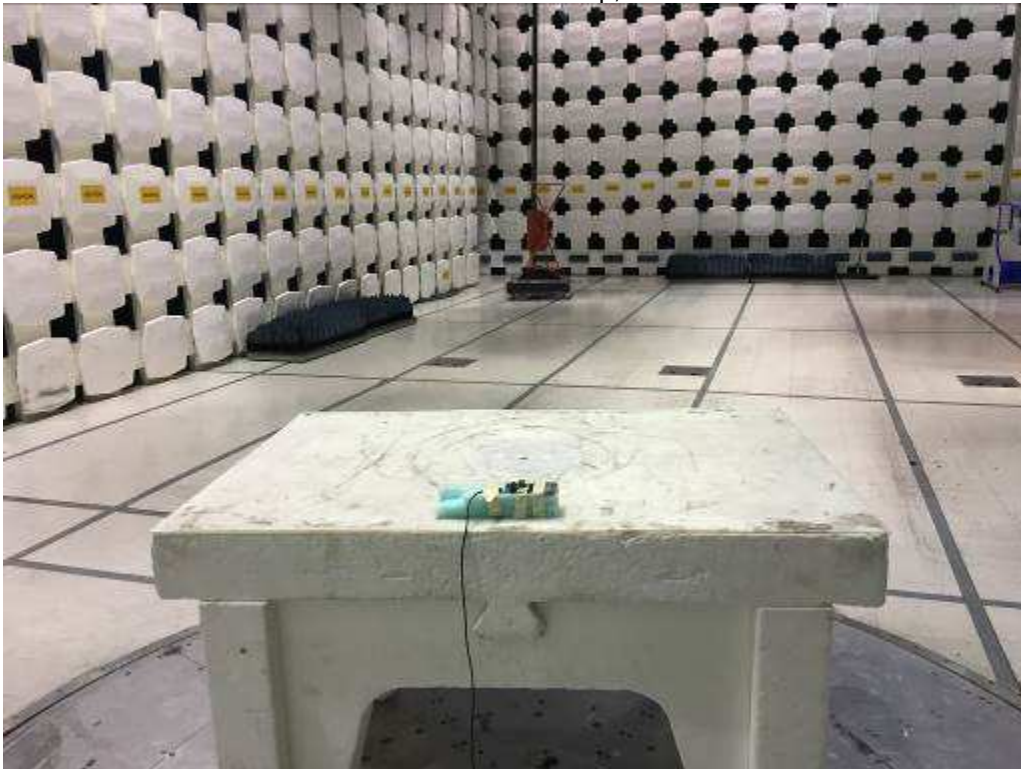
Radiated Emissions Test Setup, 30-1000 MHz
