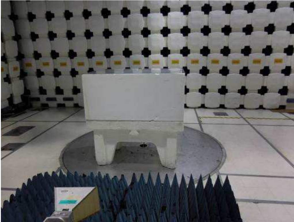
Radiated Emissions Test Setup, 1-18 GHz
