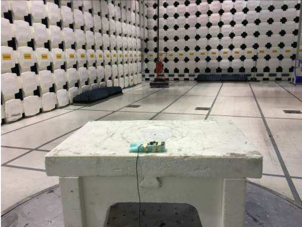
Radiated Emissions Test Setup, 30-1000 MHz
