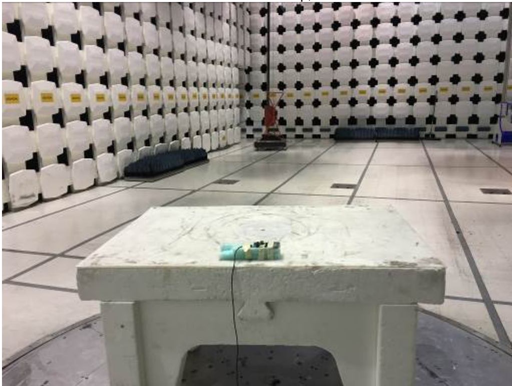
Radiated Emissions Test Setup, 30-1000 MHz
