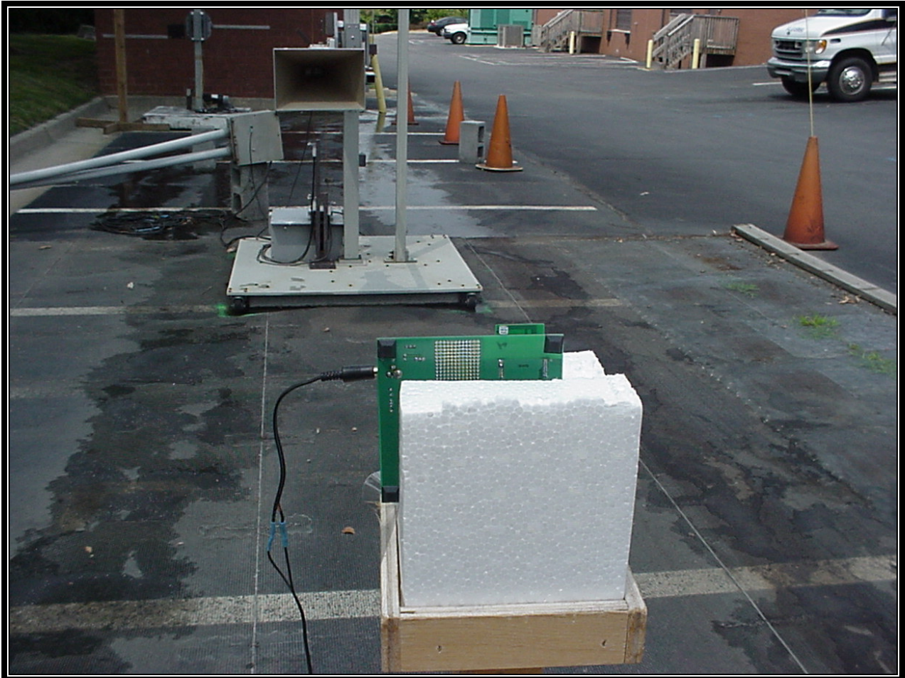
Photograph 5: Radiated Spurious/Harmonics Testing – Back View
