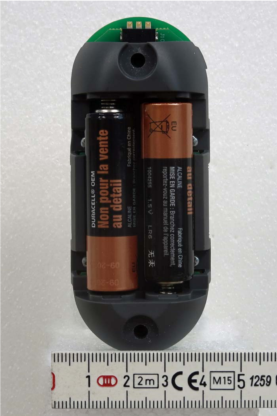
Bottom Cover Removed
