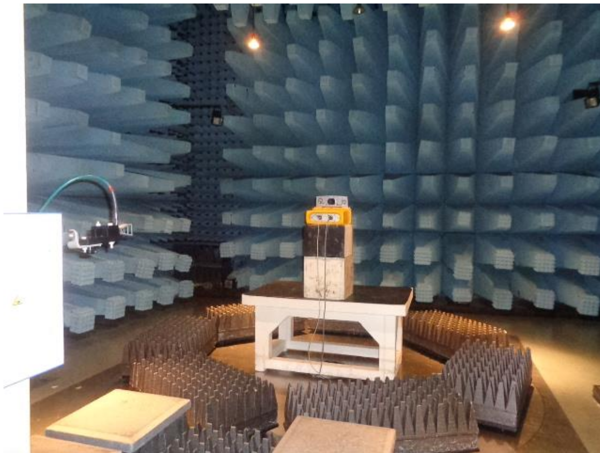
Radiated emission above 1 GHz
