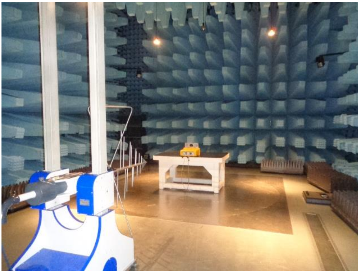
Radiated emission below 1 GHz
