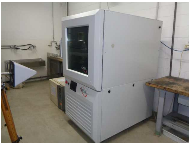
Figure 9.1-2: Antenna port testing set-up in climatic chamber
