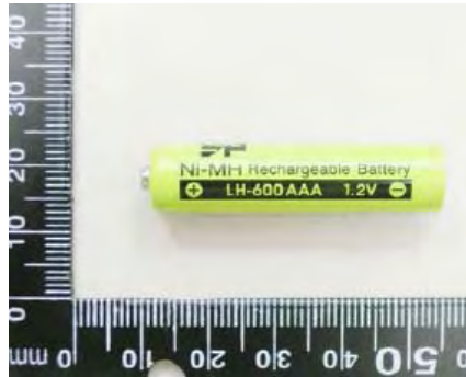
Figure 2. Battery(Ni-MH 1.2V 600mAh )
