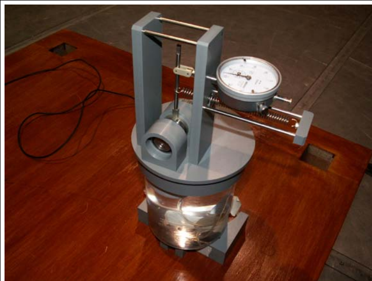
Strength test equipment, implant placed in saline solution to simulate human body.
