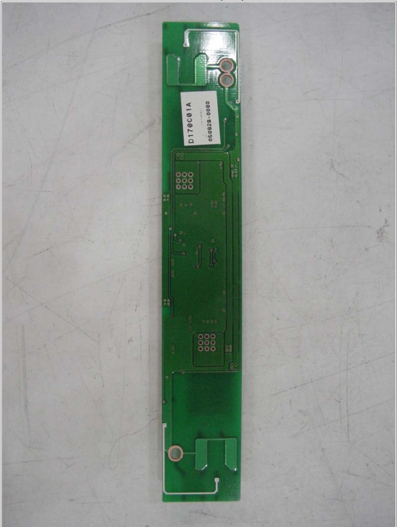
Inverter Board (Rear)
