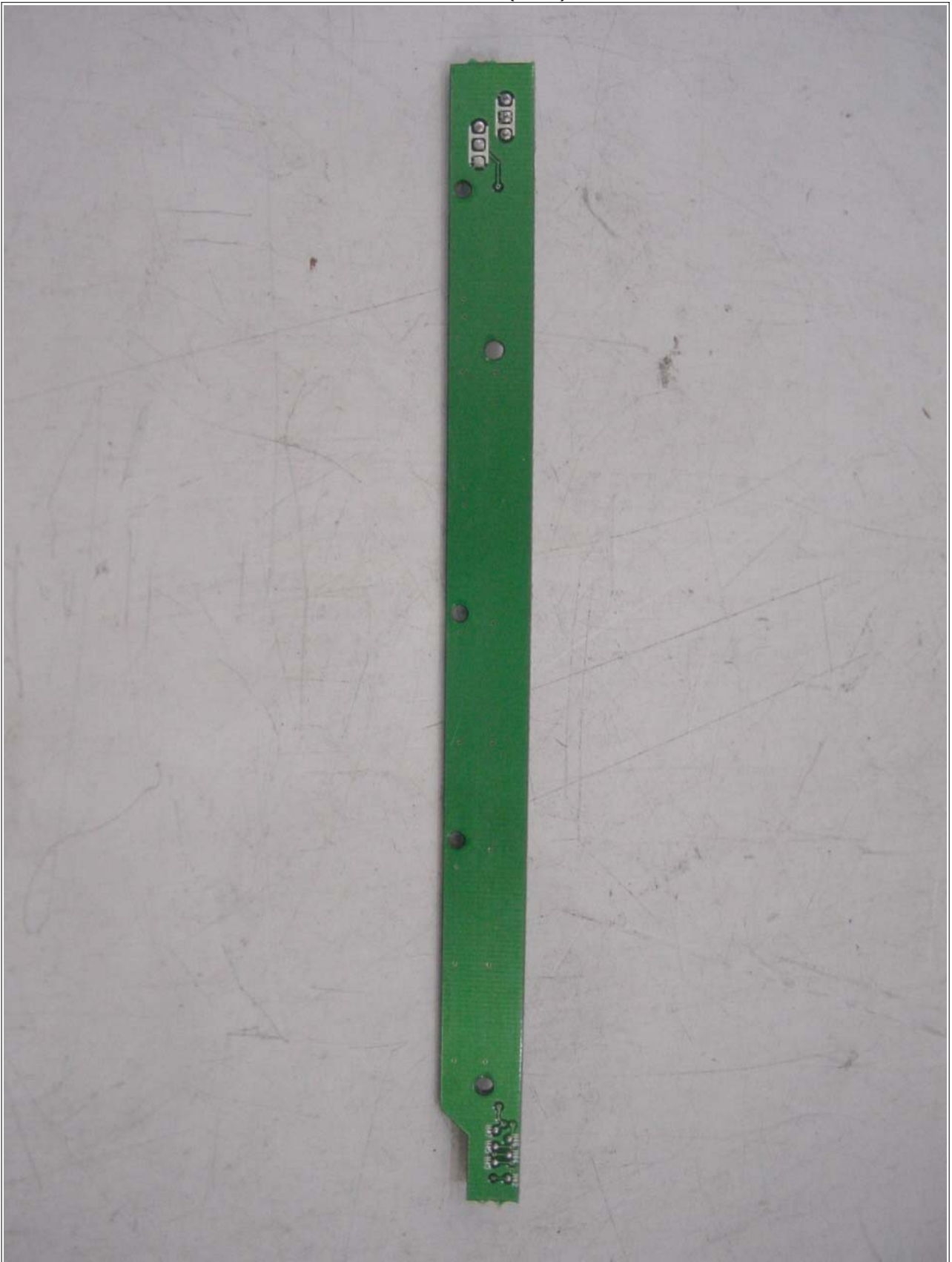
OSD Board (Rear)
