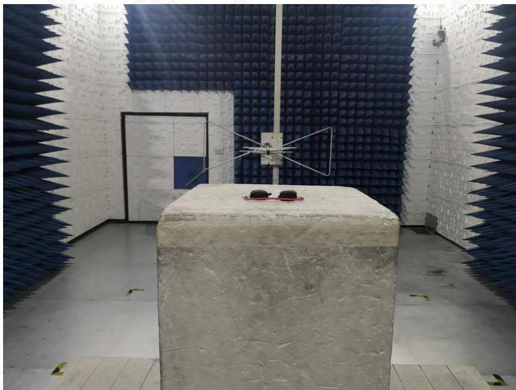
RADIATED EMISSION TEST SETUP ABOVE 1GHZ
