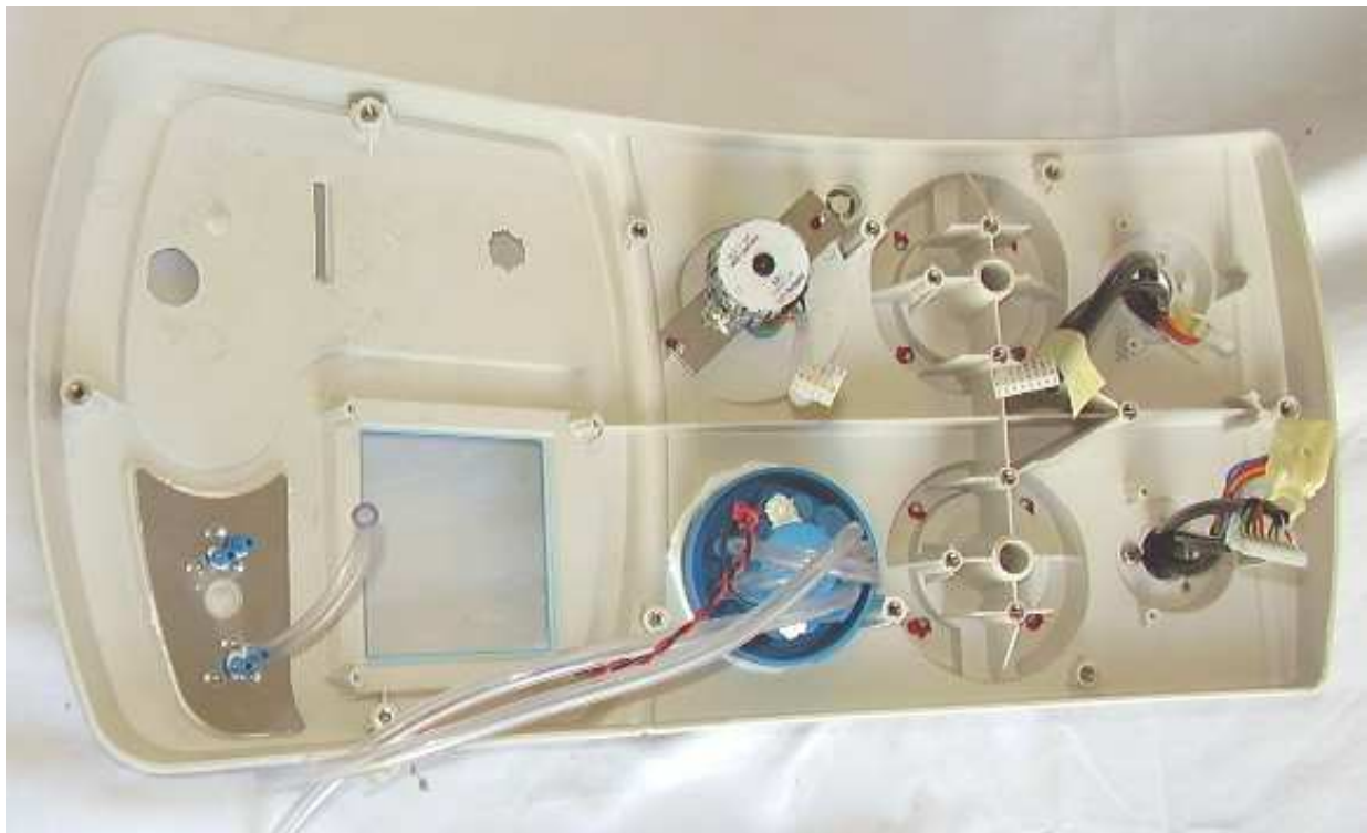
Upper face without keyboard, screen and burettes motors
