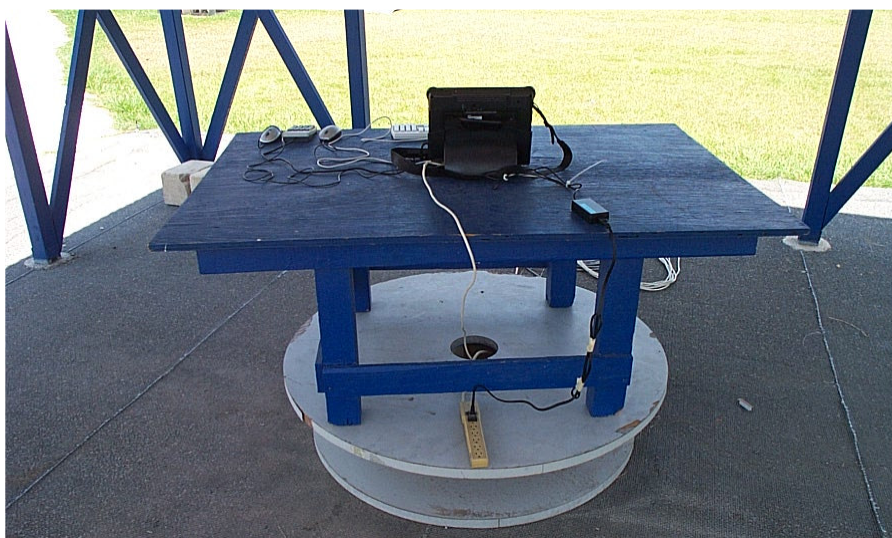
Figure 11 Spurious 30 - 1000 MHz, Cables
