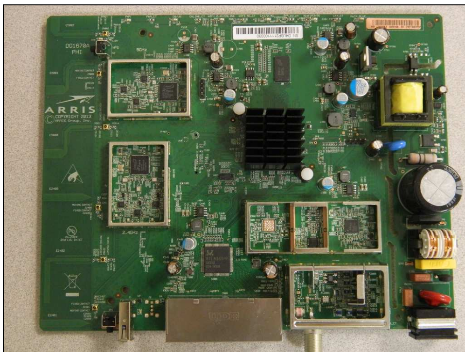
Figure 4: Internal Photo – DG1660A – Shields Removed
