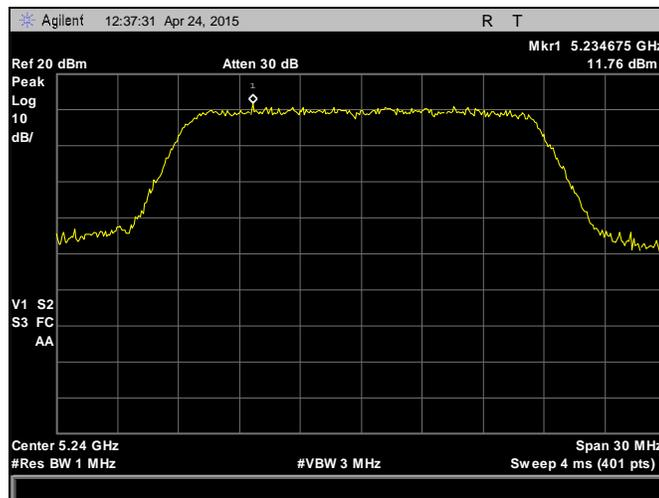
Plot 72. Peak Power Spectral Density, 5240 MHz, 802.11n, HT20, Chain 2
