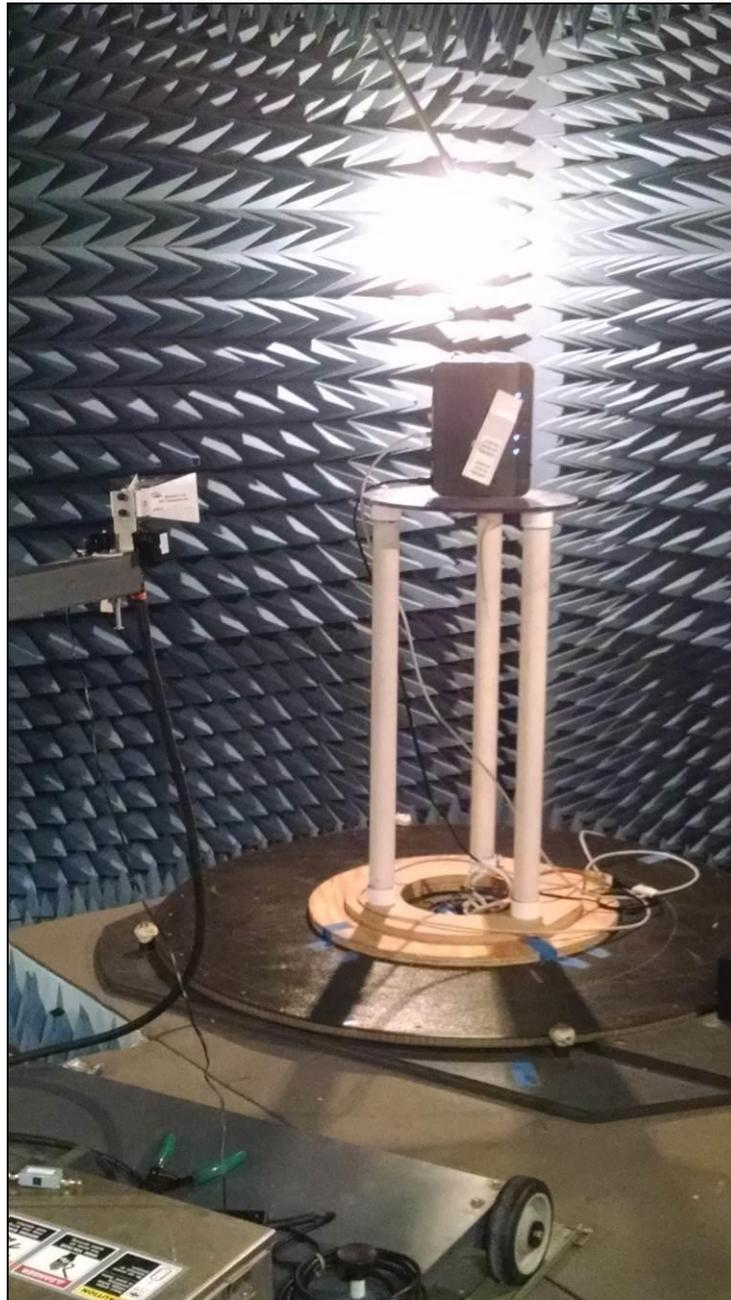
**Photograph 3. Radiated Test Setup, 18 GHz – 40 GHz**
