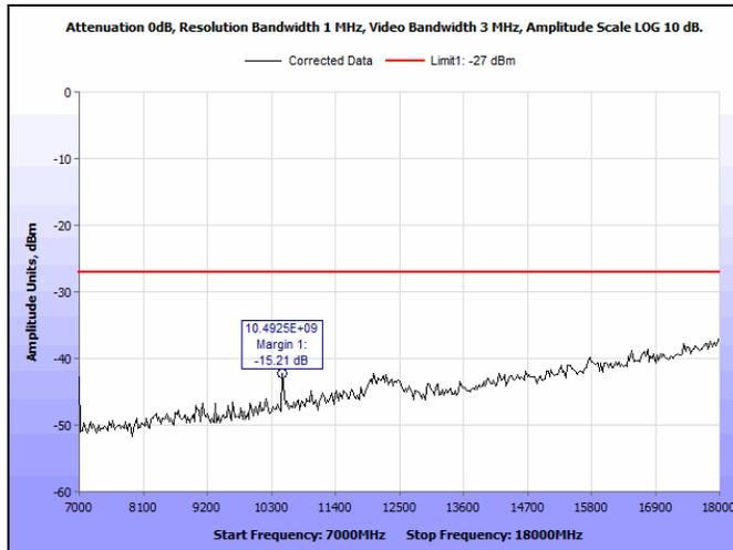
Plot 90. Radiated Spurious Emissions, 5240 MHz, 802.11a, 7 GHz – 18 GHz
