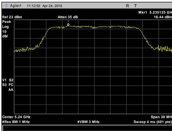
Plot 71. Peak Power Spectral Density, 5240 MHz, 802.11n, HT20, Chain 1
