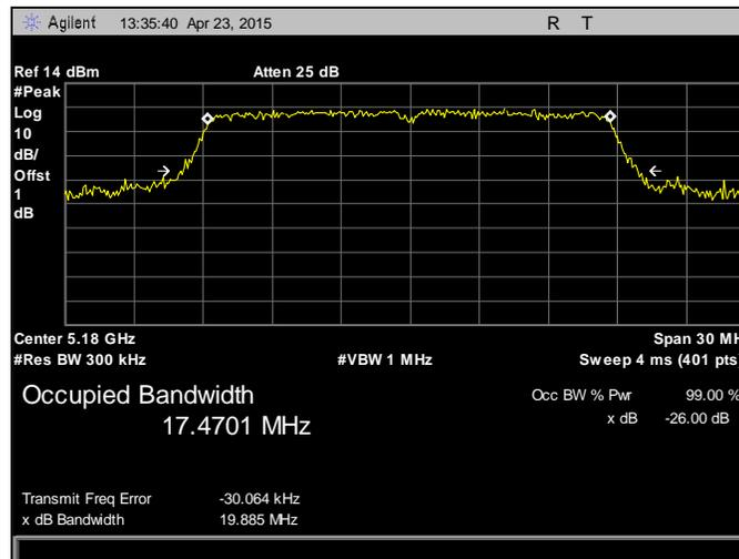
Plot 12. 26 dB Occupied Bandwidth, 5180 MHz, 802.11n, HT20, Chain 2
