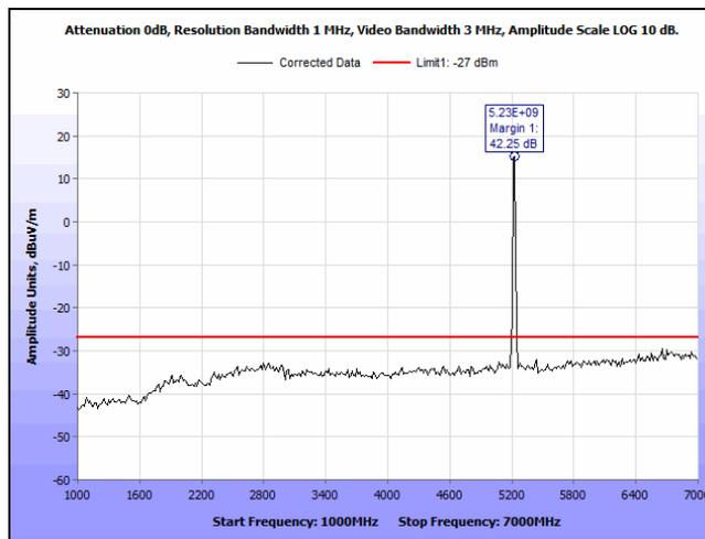
Plot 86. Radiated Spurious Emissions, 5200 MHz, 802.11a, 1 GHz – 7 GHz
