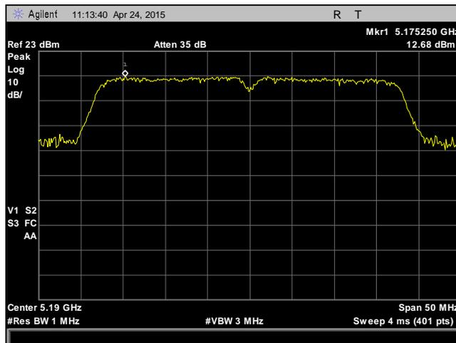
Plot 74. Peak Power Spectral Density, 5190 MHz, 802.11n, HT40, Chain 1
