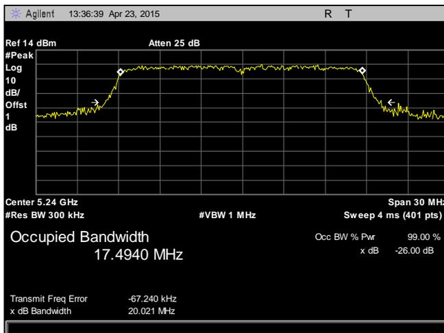
Plot 18. 26 dB Occupied Bandwidth, 5240 MHz, 802.11n, HT20, Chain 2
