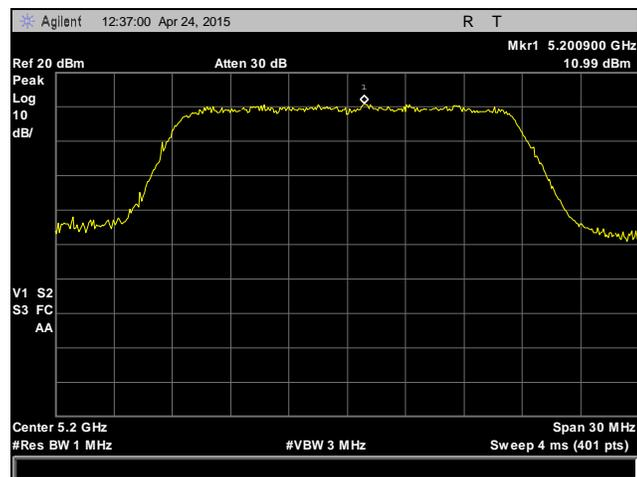
Plot 69. Peak Power Spectral Density, 5200 MHz, 802.11n, HT20, Chain 2
