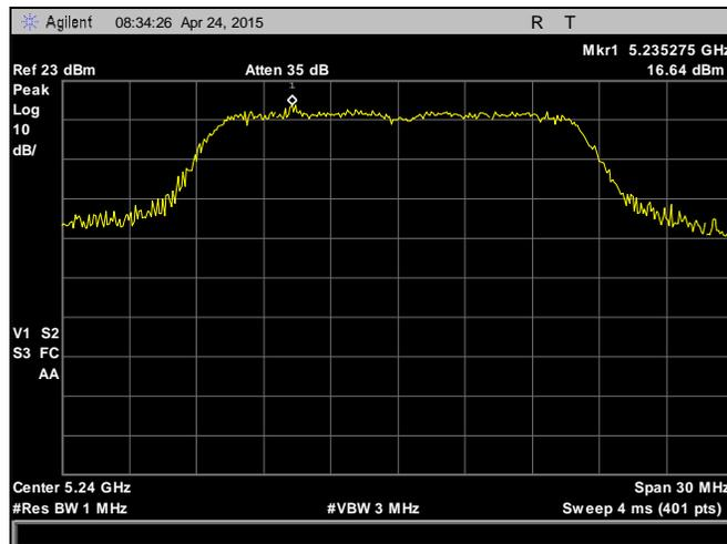
**Plot 62. Peak Power Spectral Density, 5240 MHz, 802.11a, Chain 1**
