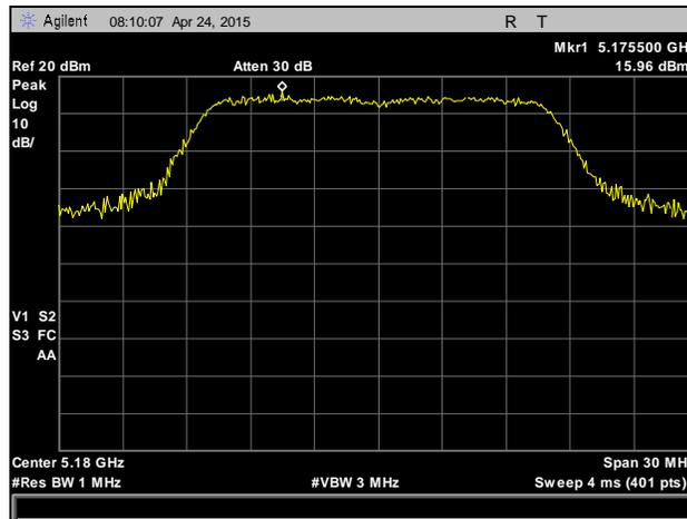
Plot 55. Peak Power Spectral Density, 5180 MHz, 802.11a, Chain 0
