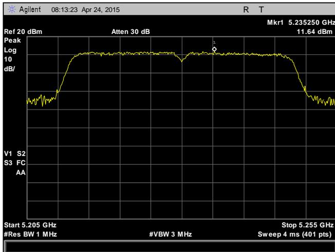
Plot 79. Peak Power Spectral Density, 5230 MHz, 802.11n, HT40, Chain 0
