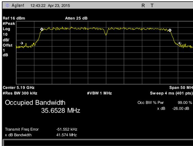
Plot 19. 26 dB Occupied Bandwidth, 5190 MHz, 802.11n, HT40, Chain 0
