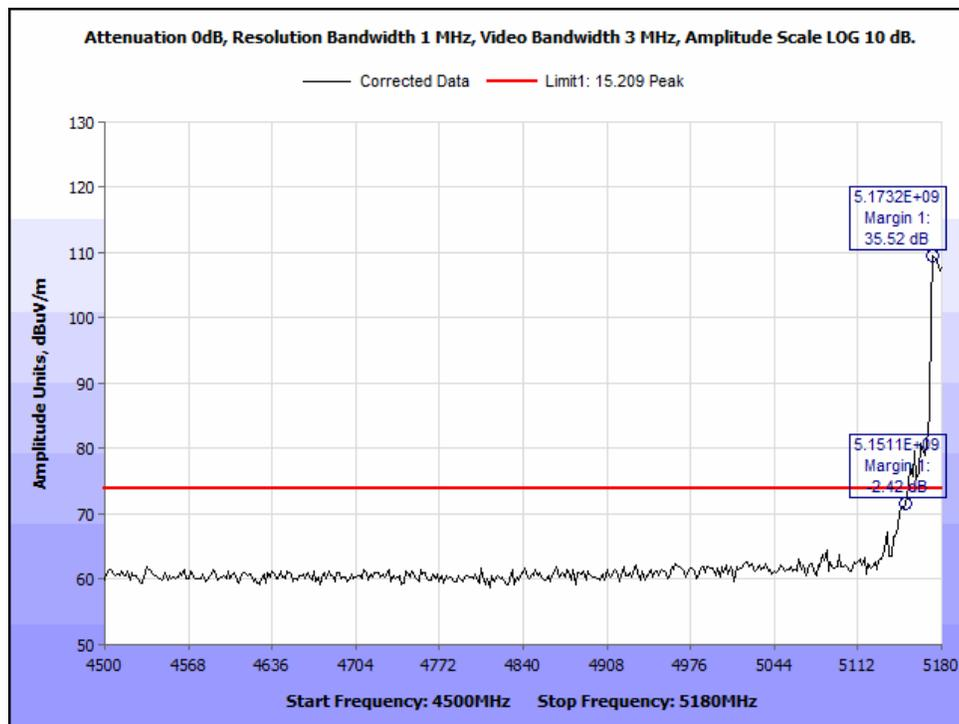
Plot 114. Radiated Band Edge, 5190 MHz, Peak, 802.11n, HT40
