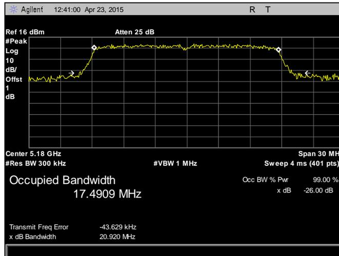
Plot 10. 26 dB Occupied Bandwidth, 5180 MHz, 802.11n, HT20, Chain 0
