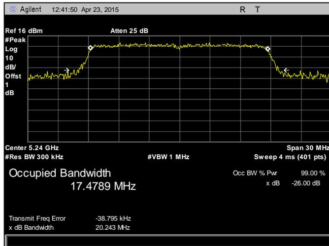
Plot 16. 26 dB Occupied Bandwidth, 5240 MHz, 802.11n, HT20, Chain 0
