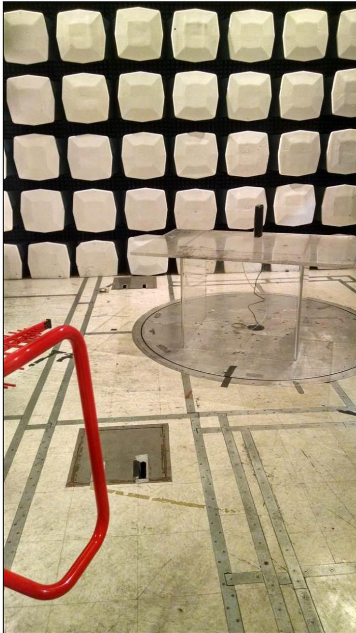
**Photograph 1. Radiated Test Setup, 30 MHz – 1 GHz**
