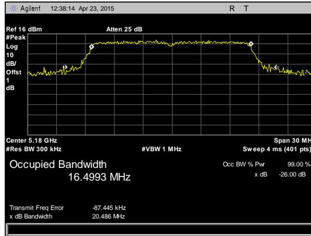
Plot 1. 26 dB Occupied Bandwidth, 5180 MHz, 802.11a, Chain 0
