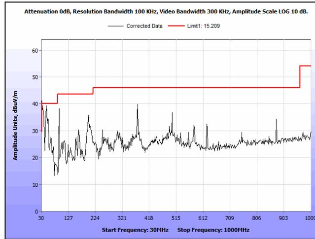
Plot 85. Radiated Spurious Emissions, 5200 MHz, 802.11a, 30 MHz – 1 GHz
