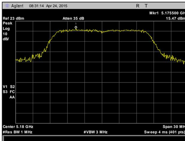
Plot 56. Peak Power Spectral Density, 5180 MHz, 802.11a, Chain 1
