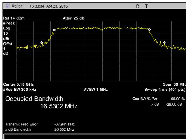
Plot 3. 26 dB Occupied Bandwidth, 5180 MHz, 802.11a, Chain 2
