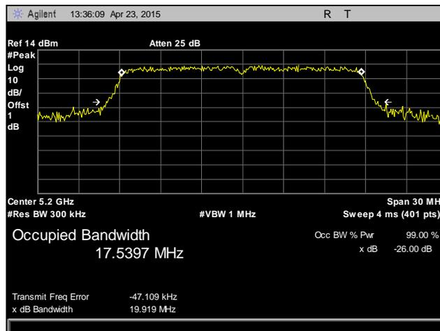
Plot 15. 26 dB Occupied Bandwidth, 5200 MHz, 802.11n, HT20, Chain 2
