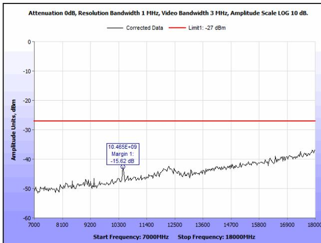
Plot 108. Radiated Spurious Emissions, 5230 MHz, 802.11n, HT40, 7 GHz – 18 GHz
