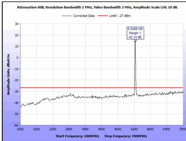
Plot 89. Radiated Spurious Emissions, 5240 MHz, 802.11a, 1 GHz – 7 GHz
