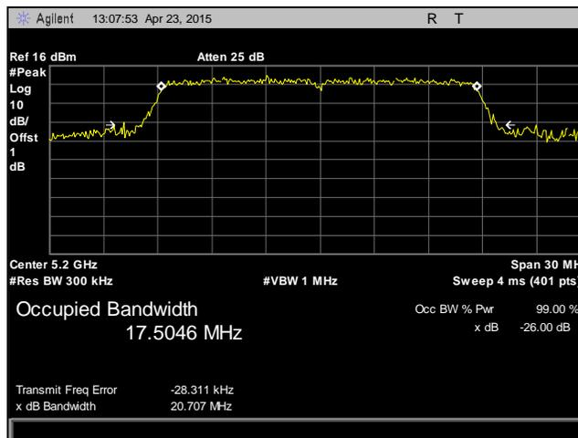
Plot 14. 26 dB Occupied Bandwidth, 5200 MHz, 802.11n, HT20, Chain 1
