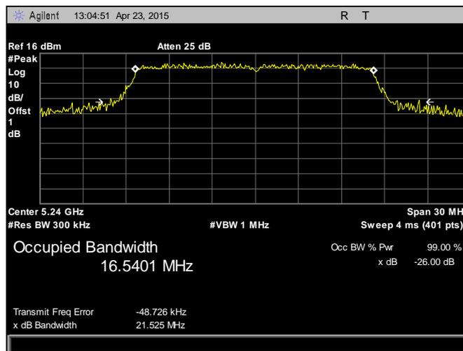
Plot 8. 26 dB Occupied Bandwidth, 5240 MHz, 802.11a, Chain 1
