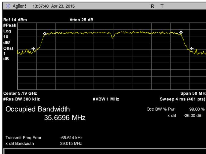
Plot 21. 26 dB Occupied Bandwidth, 5190 MHz, 802.11n, HT40, Chain 2
