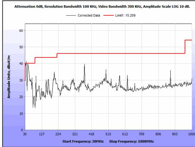
Plot 106. Radiated Spurious Emissions, 5230 MHz, 802.11n, HT40, 30 MHz – 1 GHz
