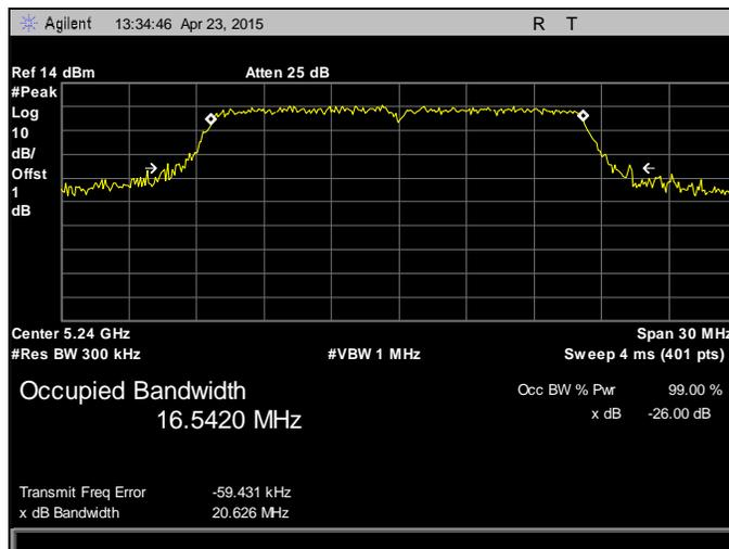
Plot 9. 26 dB Occupied Bandwidth, 5240 MHz, 802.11a, Chain 2
