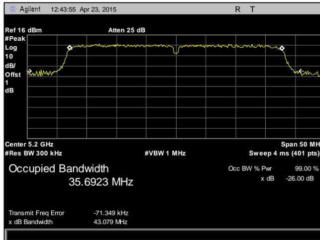
Plot 22. 26 dB Occupied Bandwidth, 5200 MHz, 802.11n, HT40, Chain 0
