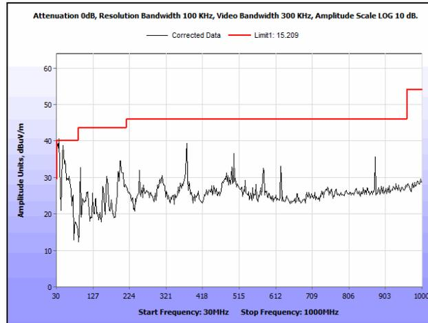
Plot 94. Radiated Spurious Emissions, 5200 MHz, 802.11n, HT20, 30 MHz – 1 GHz
