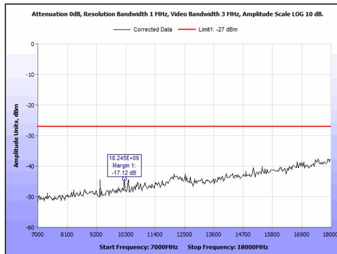
Plot 102. Radiated Spurious Emissions, 5190 MHz, 802.11n, HT40, 7 GHz – 18 GHz
