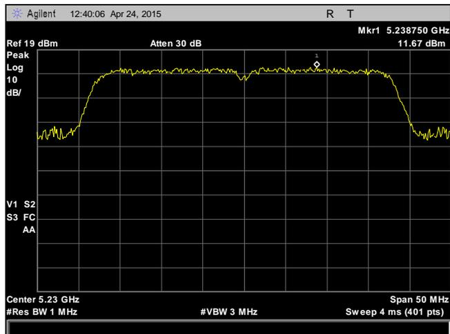
Plot 81. Peak Power Spectral Density, 5230 MHz, 802.11n, HT40, Chain 2
