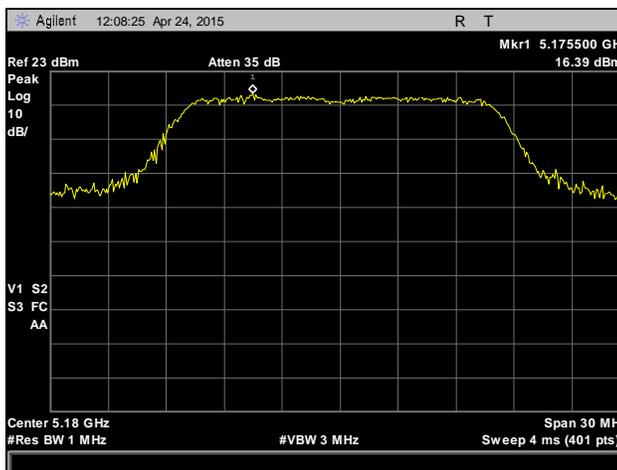
Plot 57. Peak Power Spectral Density, 5180 MHz, 802.11a, Chain 2
