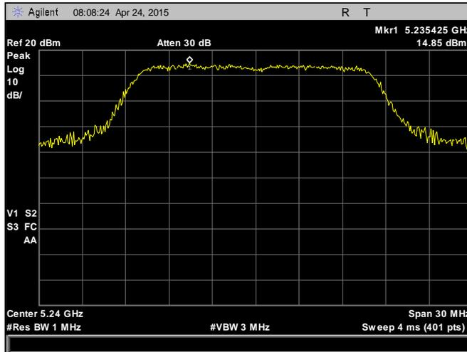
**Plot 61. Peak Power Spectral Density, 5240 MHz, 802.11a, Chain 0**
