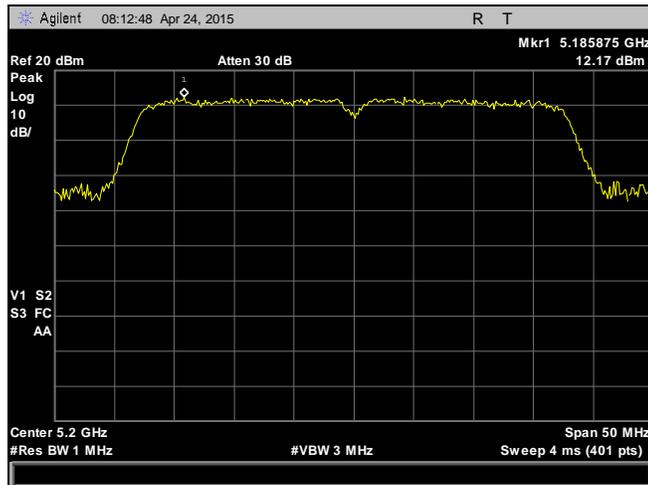
Plot 76. Peak Power Spectral Density, 5200 MHz, 802.11n, HT40, Chain 0
