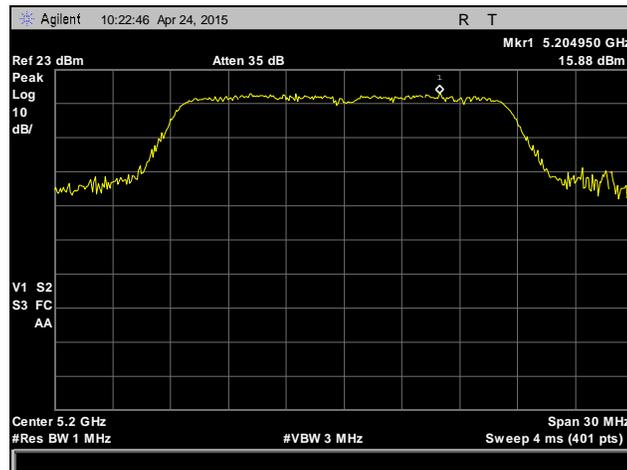
Plot 68. Peak Power Spectral Density, 5200 MHz, 802.11n, HT20, Chain 1
