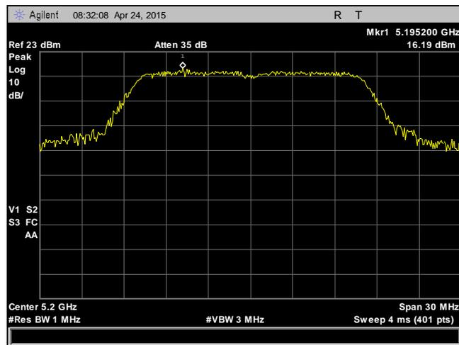
Plot 59. Peak Power Spectral Density, 5200 MHz, 802.11a, Chain 1
