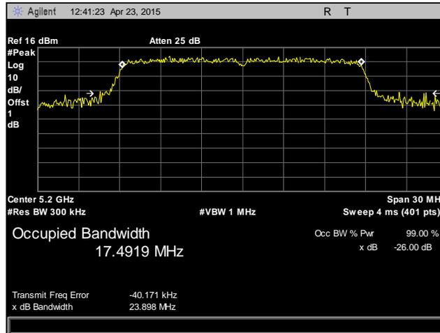
Plot 13. 26 dB Occupied Bandwidth, 5200 MHz, 802.11n, HT20, Chain 0
