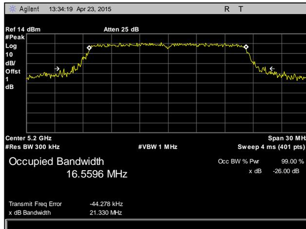
**Plot 6. 26 dB Occupied Bandwidth, 5200 MHz, 802.11a, Chain 2**
