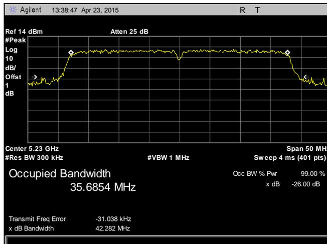
Plot 27. 26 dB Occupied Bandwidth, 5230 MHz, 802.11n, HT40, Chain 2
