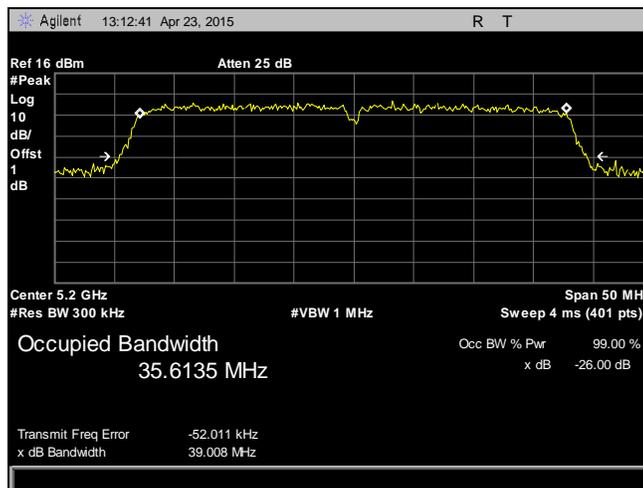
Plot 23. 26 dB Occupied Bandwidth, 5200 MHz, 802.11n, HT40, Chain 1
