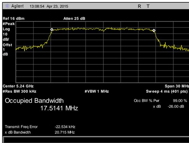
Plot 17. 26 dB Occupied Bandwidth, 5240 MHz, 802.11n, HT20, Chain 1
