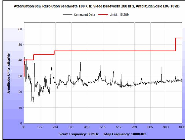
Plot 91. Radiated Spurious Emissions, 5180 MHz, 802.11n, HT20, 30 MHz – 1 GHz
