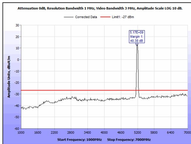
Plot 101. Radiated Spurious Emissions, 5190 MHz, 802.11n, HT40, 1 GHz – 7 GHz
