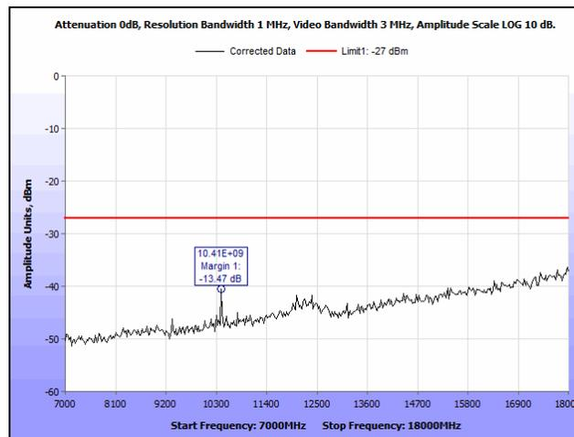
Plot 96. Radiated Spurious Emissions, 5200 MHz, 802.11n, HT20, 7 GHz – 18 GHz
