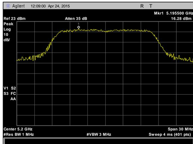
Plot 60. Peak Power Spectral Density, 5200 MHz, 802.11a, Chain 2
