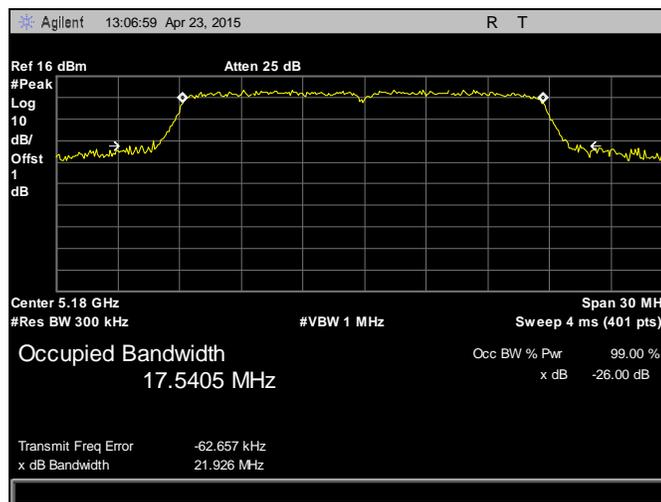
Plot 11. 26 dB Occupied Bandwidth, 5180 MHz, 802.11n, HT20, Chain 1
