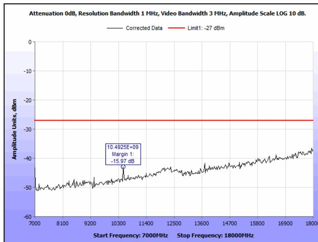
**Plot 99. Radiated Spurious Emissions, 5240 MHz, 802.11n, HT20, 7 GHz – 18 GHz**
