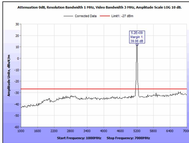
Plot 104. Radiated Spurious Emissions, 5200 MHz, 802.11n, HT40, 1 GHz – 7 GHz
