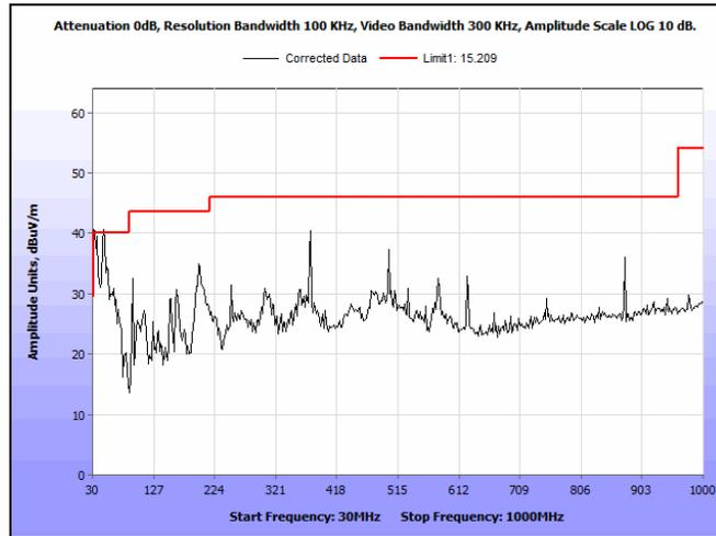
Plot 100. Radiated Spurious Emissions, 5190 MHz, 802.11n, HT40, 30 MHz – 1 GHz
