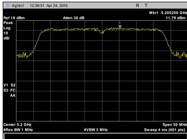
Plot 78. Peak Power Spectral Density, 5200 MHz, 802.11n, HT40, Chain 2
