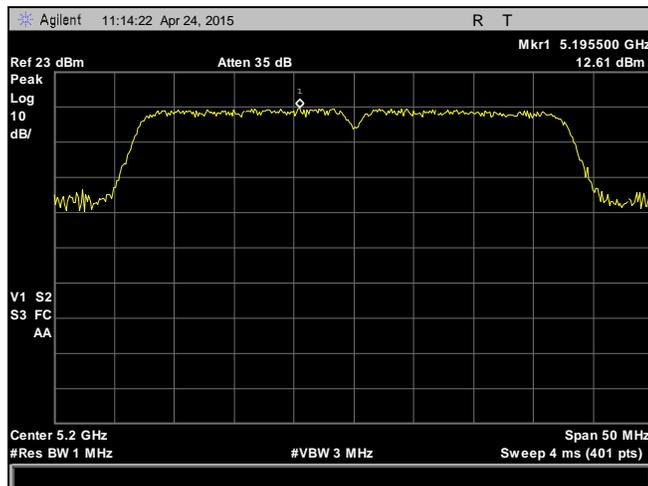
Plot 77. Peak Power Spectral Density, 5200 MHz, 802.11n, HT40, Chain 1
