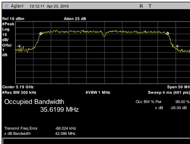
Plot 20. 26 dB Occupied Bandwidth, 5190 MHz, 802.11n, HT40, Chain 1
