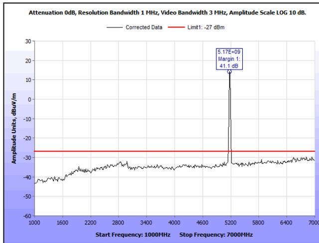
Plot 92. Radiated Spurious Emissions, 5180 MHz, 802.11n, HT20, 1 GHz – 7 GHz
