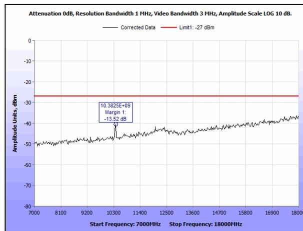
Plot 84. Radiated Spurious Emissions, 5180 MHz, 802.11a, 7 GHz – 18 GHz
