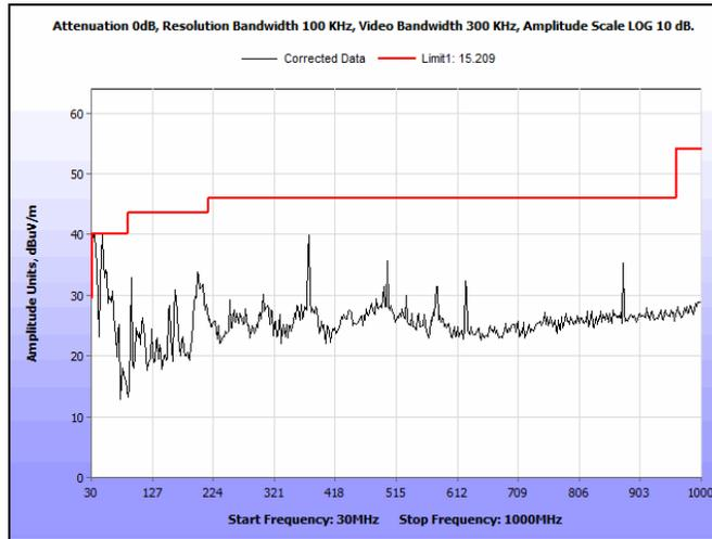
Plot 103. Radiated Spurious Emissions, 5200 MHz, 802.11n, HT40, 30 MHz – 1 GHz
