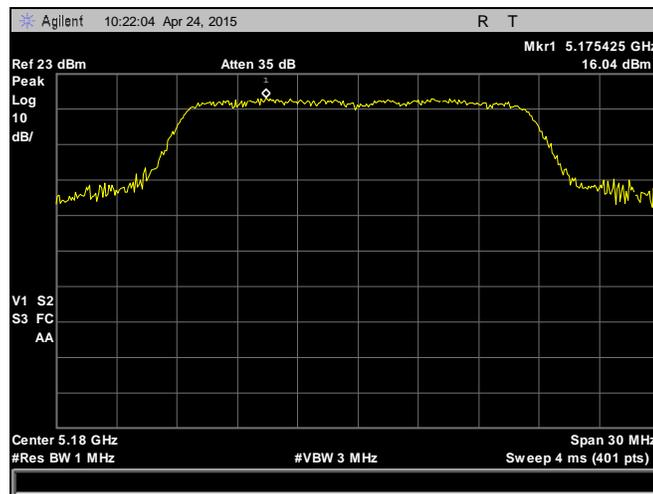
Plot 65. Peak Power Spectral Density, 5180 MHz, 802.11n, HT20, Chain 1
