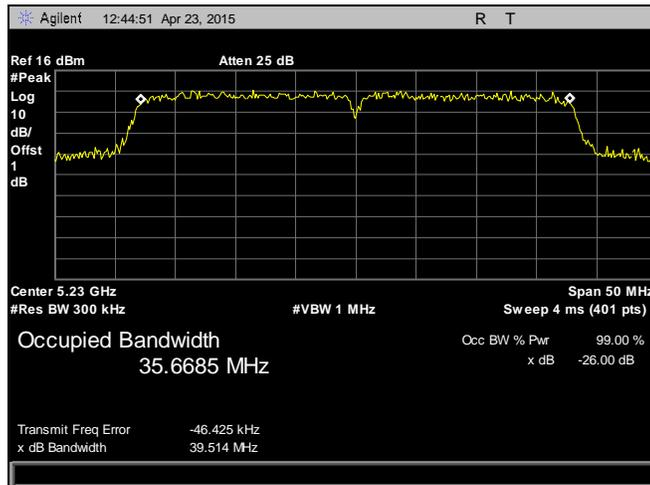
Plot 25. 26 dB Occupied Bandwidth, 5230 MHz, 802.11n, HT40, Chain 0
