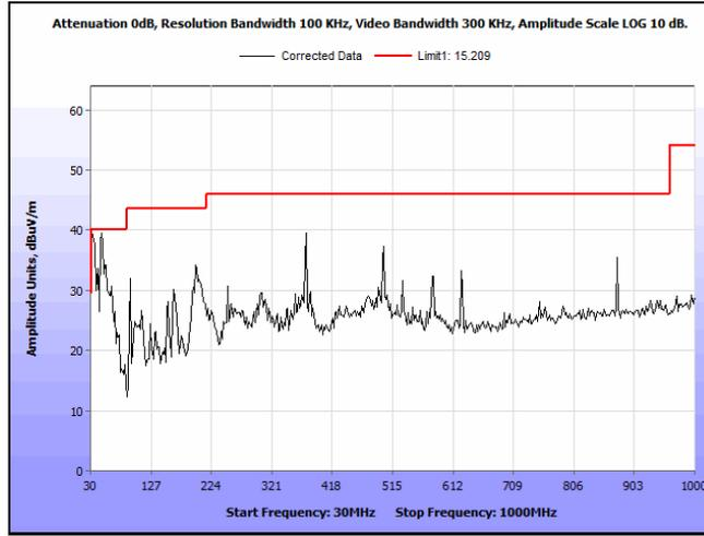
**Plot 97. Radiated Spurious Emissions, 5240 MHz, 802.11n, HT20, 30 MHz – 1 GHz**
