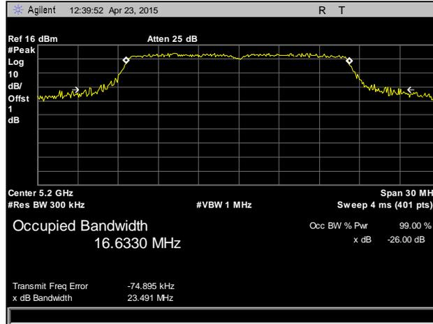
**Plot 4. 26 dB Occupied Bandwidth, 5200 MHz, 802.11a, Chain 0**
