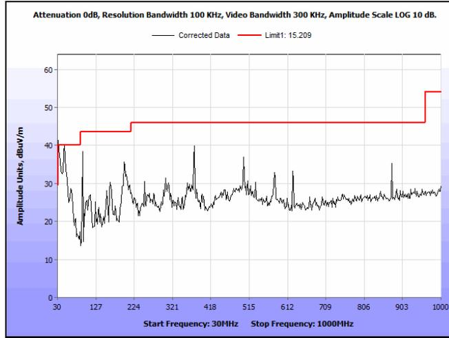
Plot 88. Radiated Spurious Emissions, 5240 MHz, 802.11a, 30 MHz – 1 GHz
