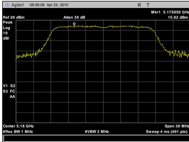
Plot 58. Peak Power Spectral Density, 5200 MHz, 802.11a, Chain 0
