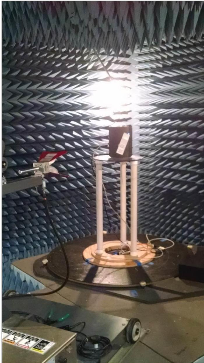
**Photograph 2. Radiated Test Setup, 1 GHz – 18 GHz**
