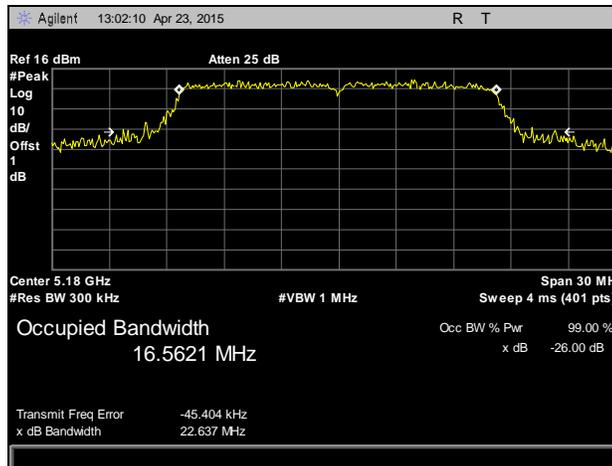
Plot 2. 26 dB Occupied Bandwidth, 5180 MHz, 802.11a, Chain 1
