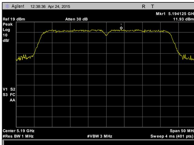
Plot 75. Peak Power Spectral Density, 5190 MHz, 802.11n, HT40, Chain 2
