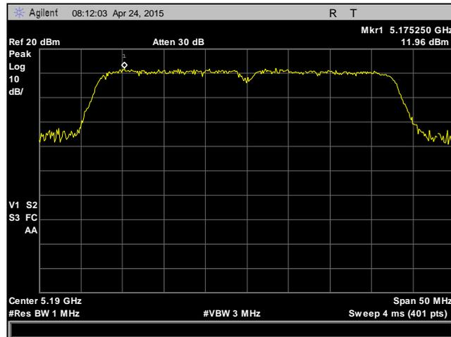
Plot 73. Peak Power Spectral Density, 5190 MHz, 802.11n, HT40, Chain 0
