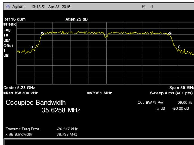
Plot 26. 26 dB Occupied Bandwidth, 5230 MHz, 802.11n, HT40, Chain 1
