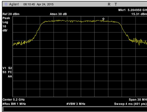
Plot 67. Peak Power Spectral Density, 5200 MHz, 802.11n, HT20, Chain 0
