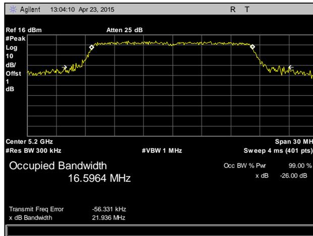
**Plot 5. 26 dB Occupied Bandwidth, 5200 MHz, 802.11a, Chain 1**
