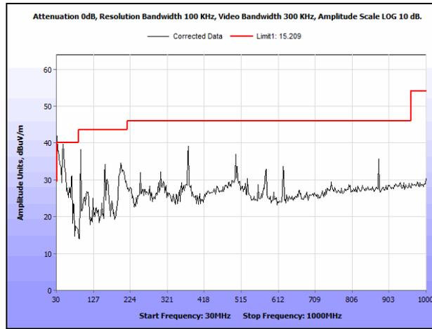
Plot 82. Radiated Spurious Emissions, 5180 MHz, 802.11a, 30 MHz – 1 GHz
