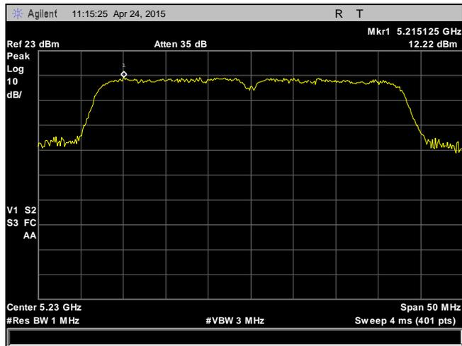
Plot 80. Peak Power Spectral Density, 5230 MHz, 802.11n, HT40, Chain 1
