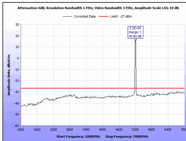
Plot 95. Radiated Spurious Emissions, 5200 MHz, 802.11n, HT20, 1 GHz – 7 GHz
