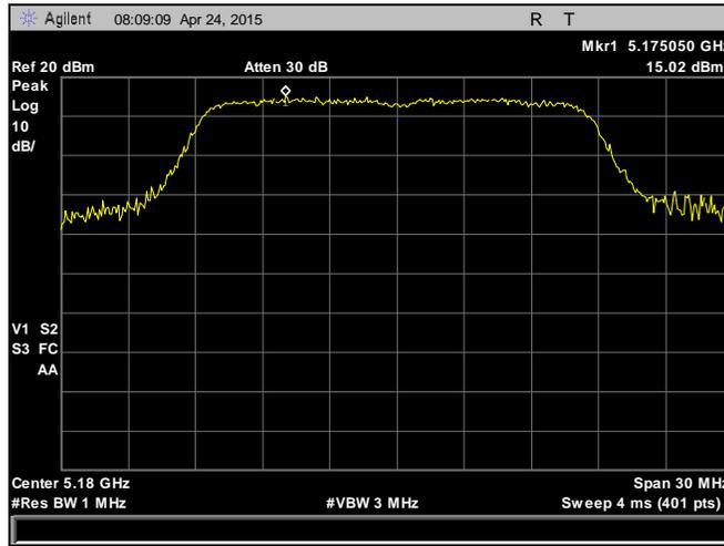
Plot 64. Peak Power Spectral Density, 5180 MHz, 802.11n, HT20, Chain 0
