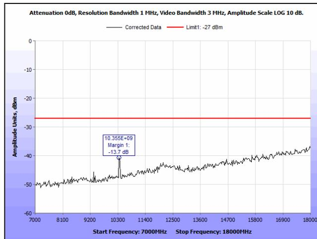
Plot 93. Radiated Spurious Emissions, 5180 MHz, 802.11n, HT20, 7 GHz – 18 GHz
