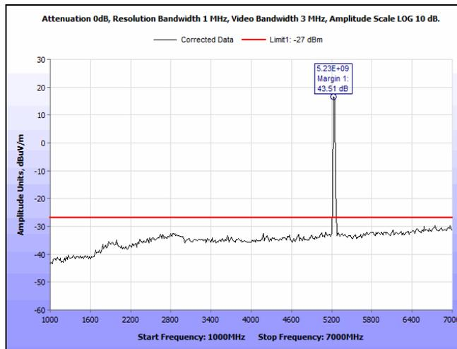
**Plot 98. Radiated Spurious Emissions, 5240 MHz, 802.11n, HT20, 1 GHz – 7 GHz**
