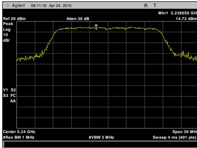
Plot 70. Peak Power Spectral Density, 5240 MHz, 802.11n, HT20, Chain 0
