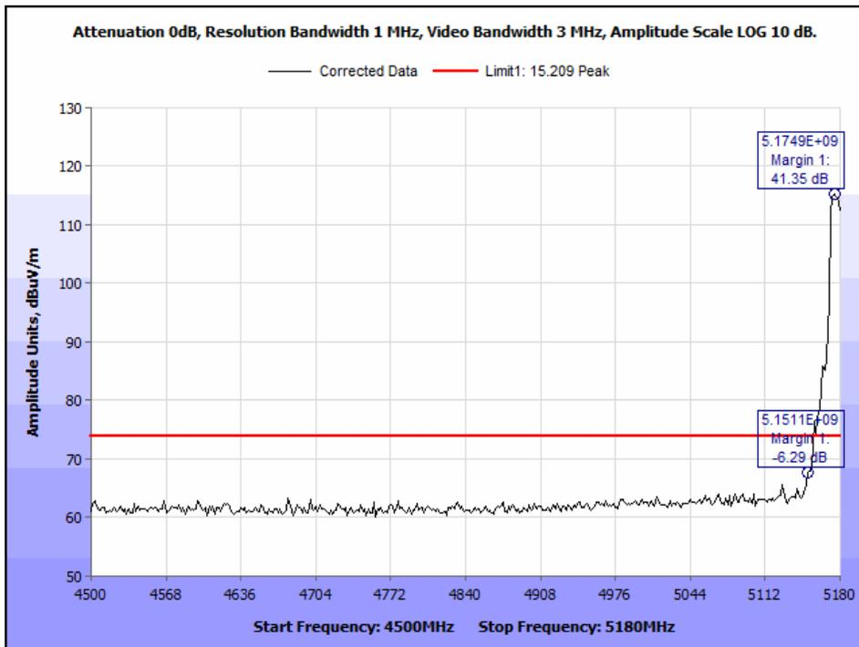
Plot 112. Radiated Band Edge, 5180 MHz, Peak, 802.11n, HT20
