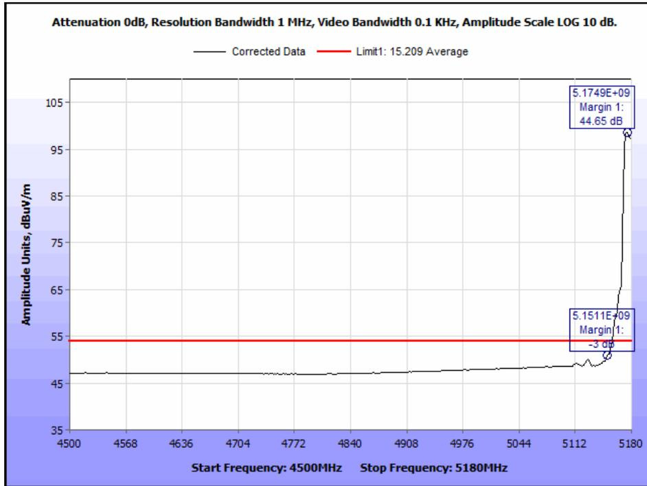
Plot 111. Radiated Band Edge, 5180 MHz, Average, 802.11n, HT20
