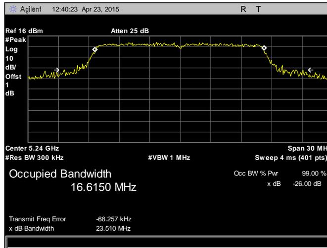
Plot 7. 26 dB Occupied Bandwidth, 5240 MHz, 802.11a, Chain 0
