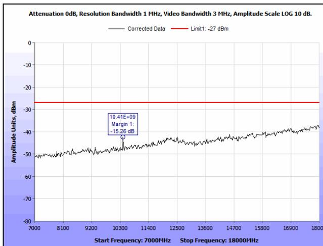
Plot 87. Radiated Spurious Emissions, 5200 MHz, 802.11a, 7 GHz – 18 GHz
