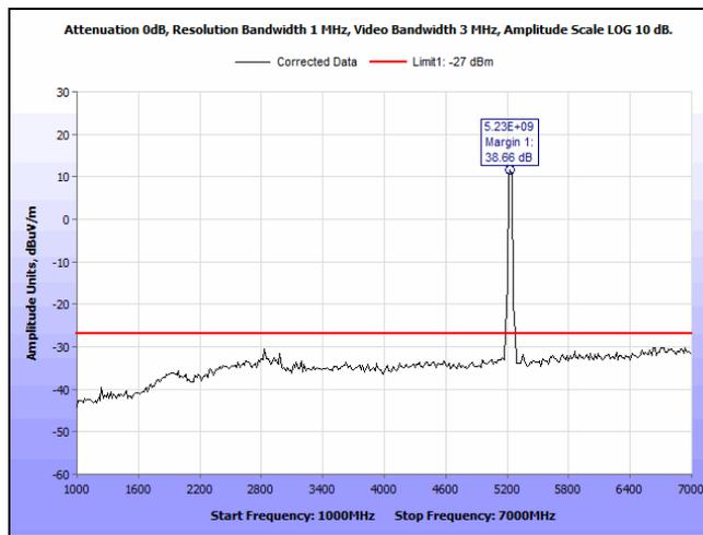
Plot 107. Radiated Spurious Emissions, 5230 MHz, 802.11n, HT40, 1 GHz – 7 GHz
