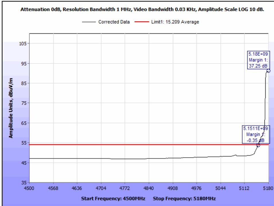
Plot 113. Radiated Band Edge, 5190 MHz, Average, 802.11n, HT40
