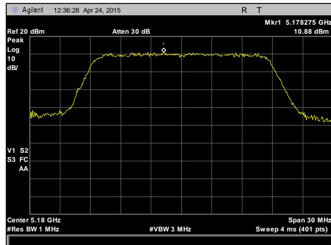
Plot 66. Peak Power Spectral Density, 5180 MHz, 802.11n, HT20, Chain 2
