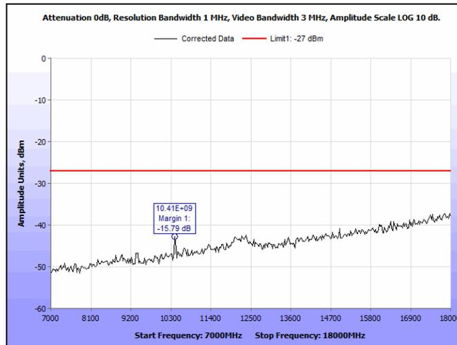
Plot 105. Radiated Spurious Emissions, 5200 MHz, 802.11n, HT40, 7 GHz – 18 GHz
