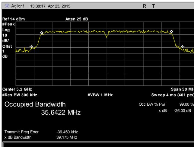
Plot 24. 26 dB Occupied Bandwidth, 5200 MHz, 802.11n, HT40, Chain 2
