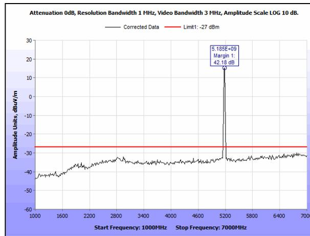
Plot 83. Radiated Spurious Emissions, 5180 MHz, 802.11a, 1 GHz – 7 GHz
