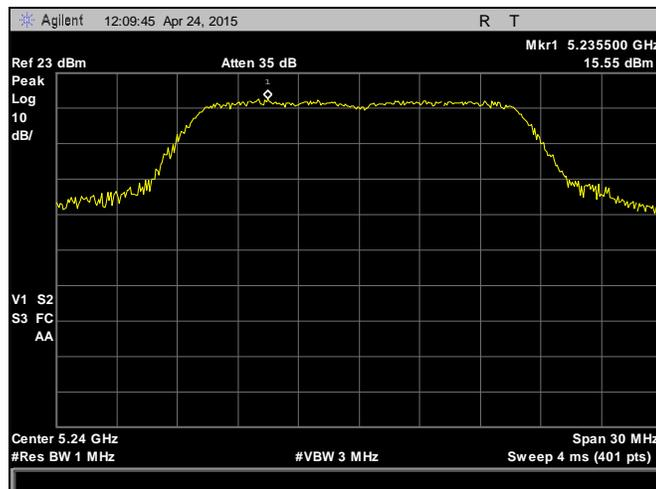
**Plot 63. Peak Power Spectral Density, 5240 MHz, 802.11a, Chain 2**
