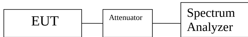
Figure 2. Power Output Test Setup
