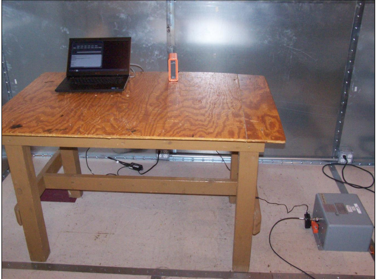
Photograph 1. Conducted Emissions, 15.207(a), Test Setup
