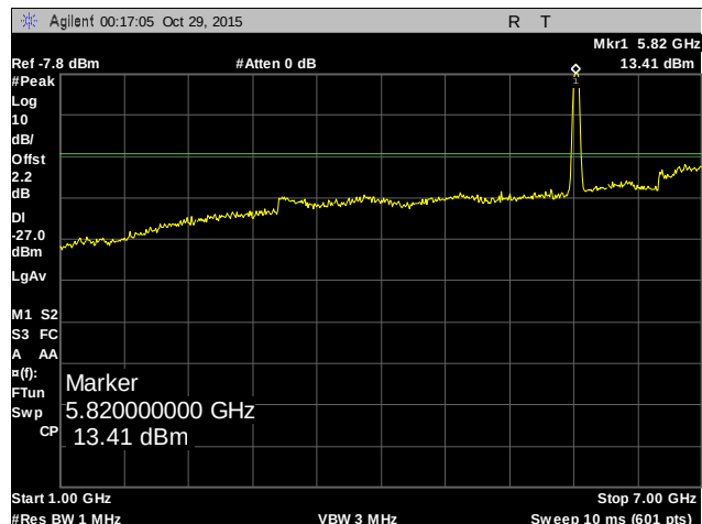
Plot 75. Radiated Spurious Emissions, Above 1 GHz, High Channel, 802.11a
