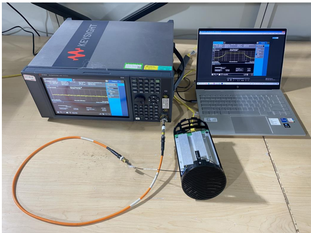
Description: 6GHz RLAN RF Conducted Test Setup
