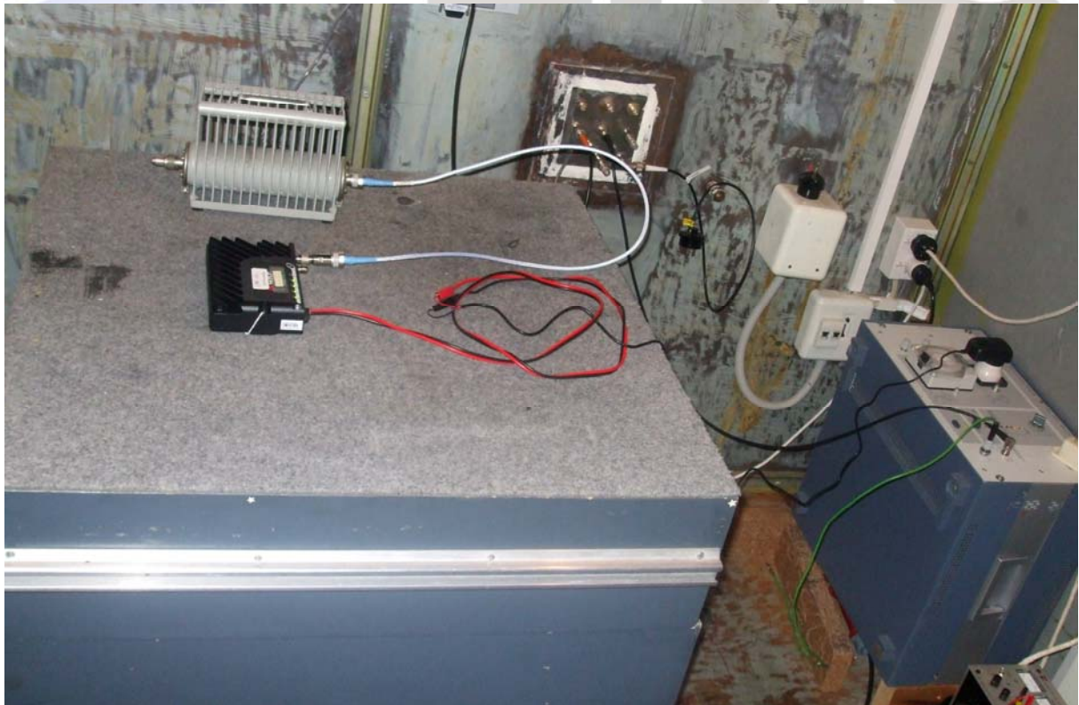
Conducted emissions setup
