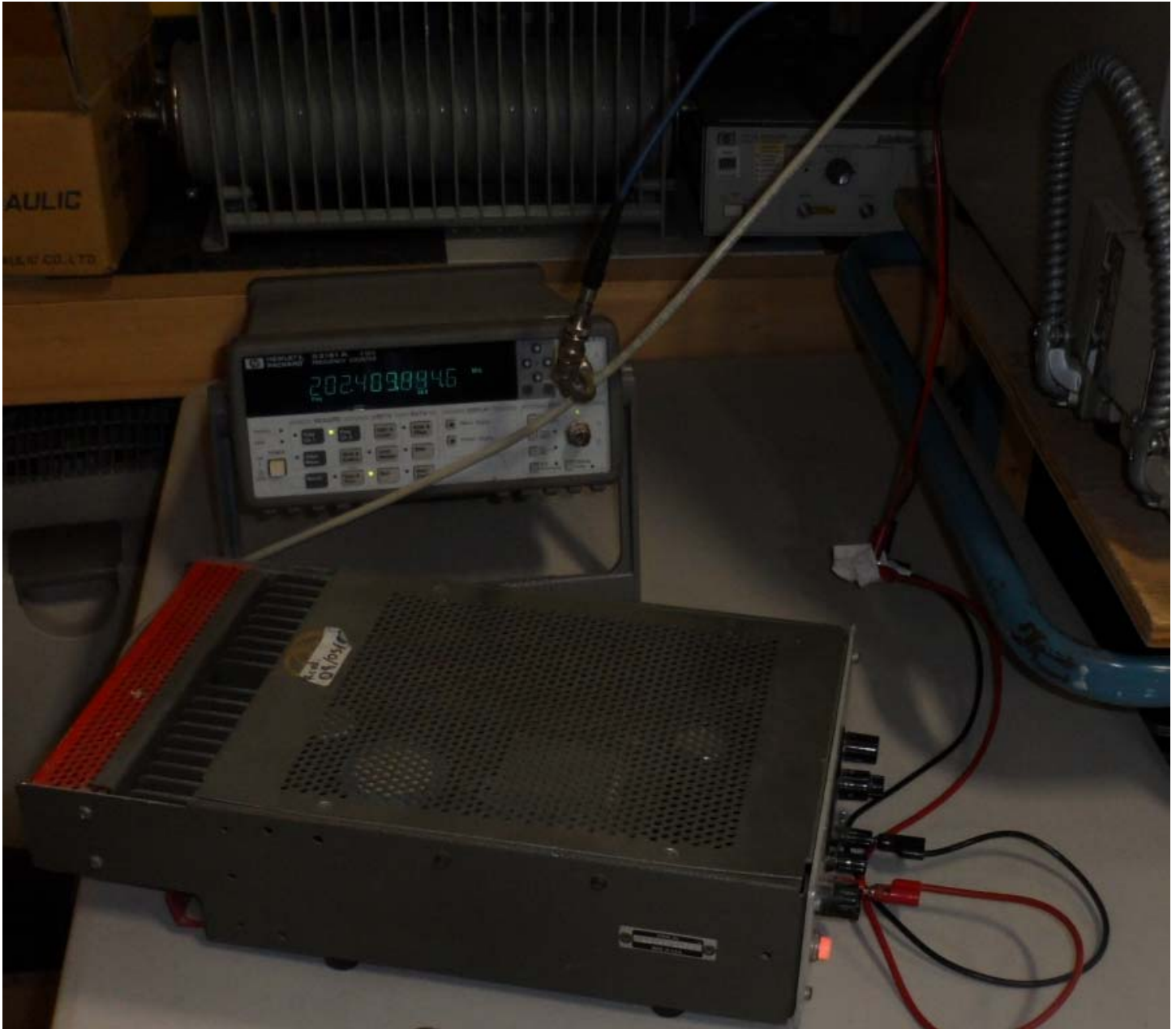
Figure E15.2 – Setup Photo – Frequency Stability Equipment
