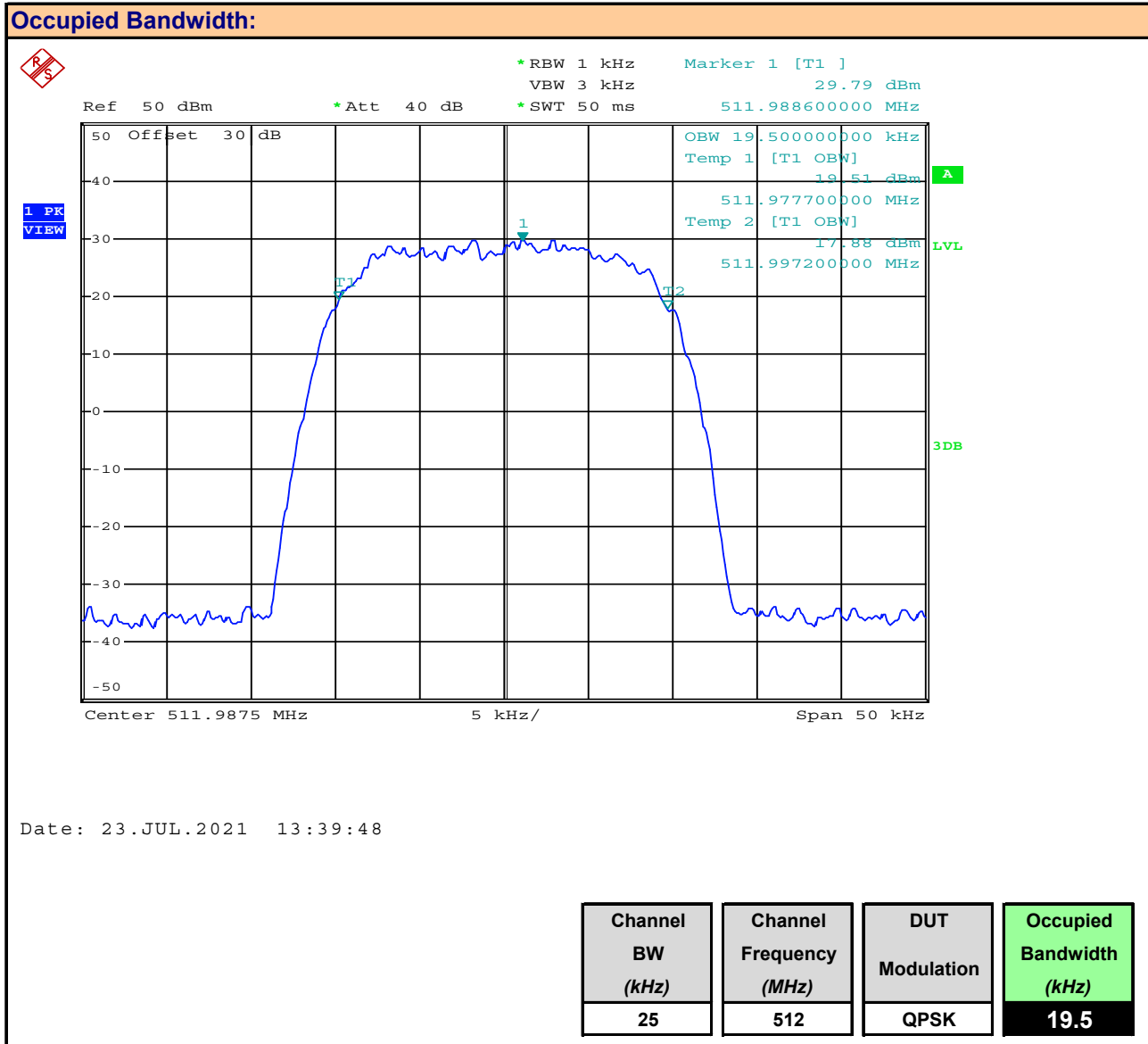
Plot 8.12 – Occupied Bandwidth, 25kHz BW, 512MHz, QPSK
