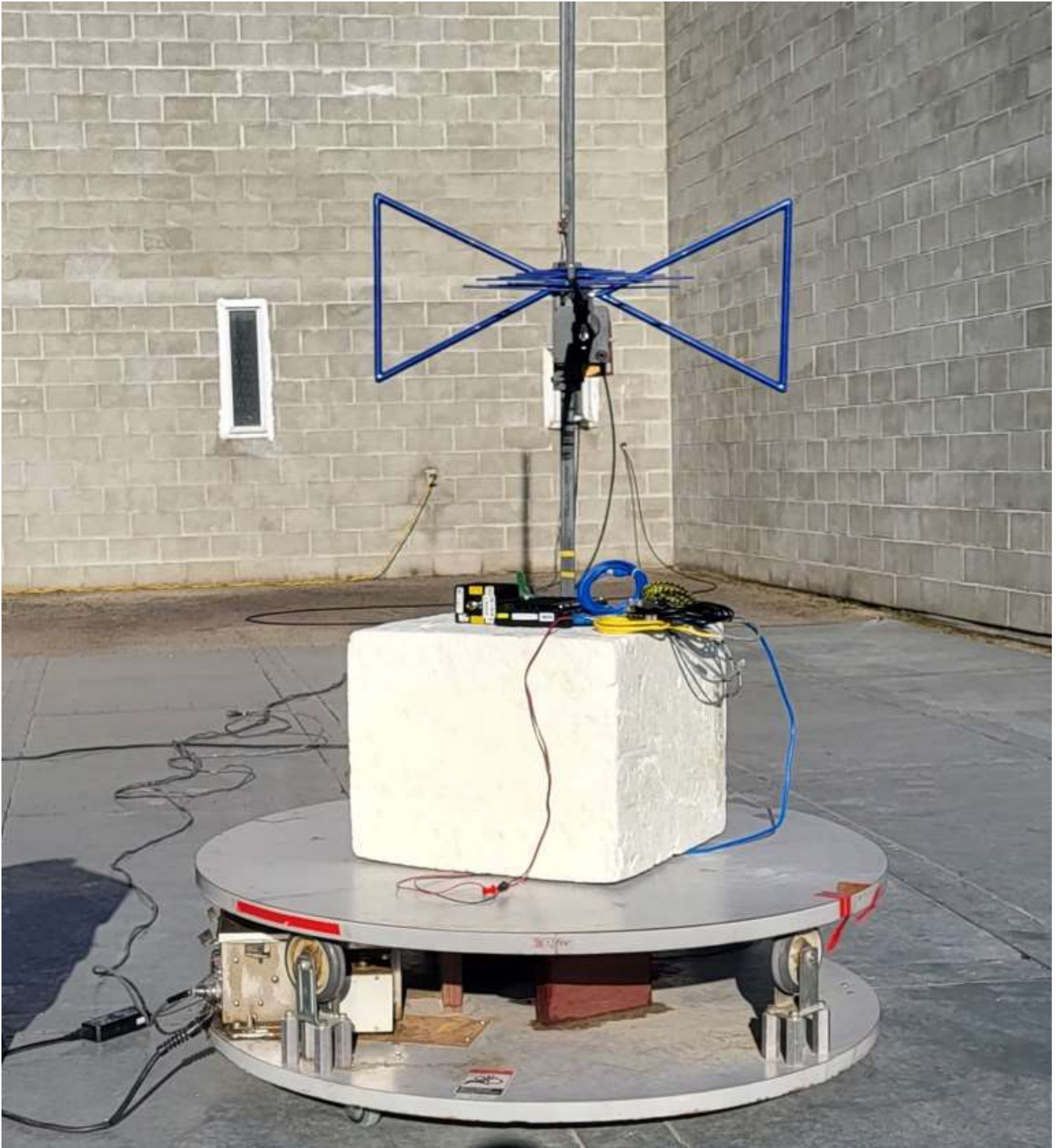
Figure E12.4 – Setup, Radiated Rx Measurements, 30-1000MHz, with Cabling
