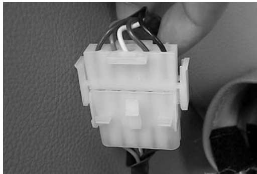
Figure 15 The amplifier power cable (5 pin) connects to the 5 pin amplifier power cable originating at the left rear of the seat frame.
