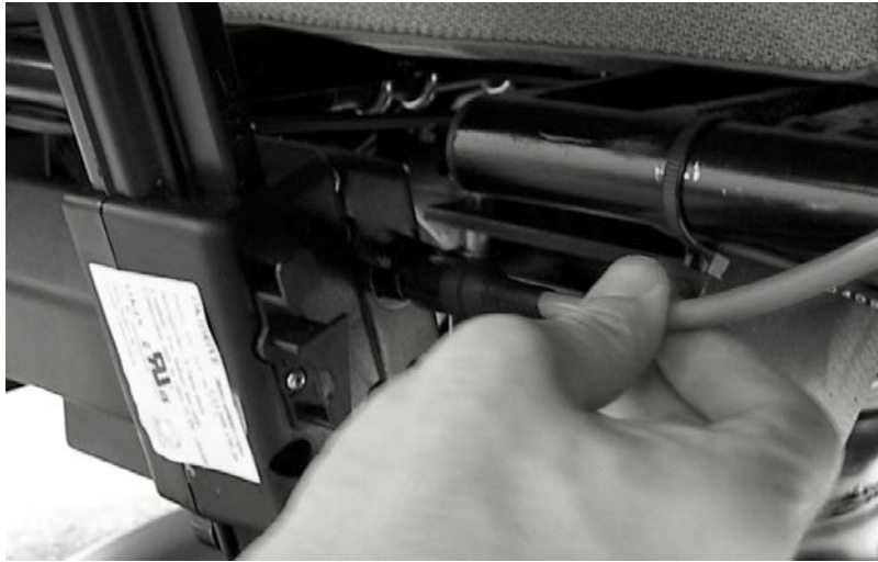
Figure 9 The recline control cable exiting the right arm connects directly to the recline motor.
