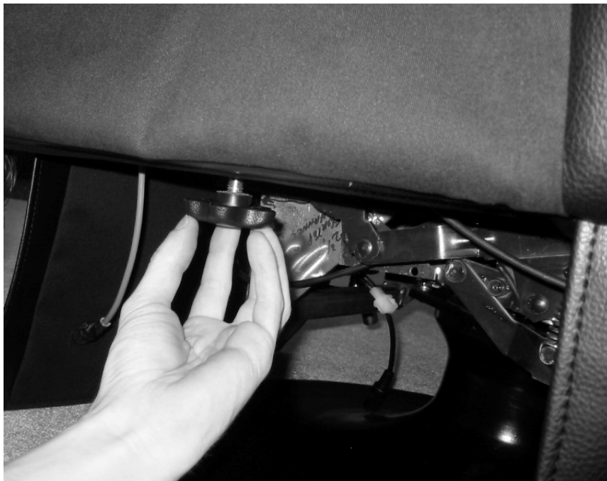
Figure 8 The right arm assembly is being held on top of the right side L-bracket and is positioned properly so that the holes in the bottom of the arm assembly match the holes in the L-bracket so that the hand-bolts can be inserted and tightened.
