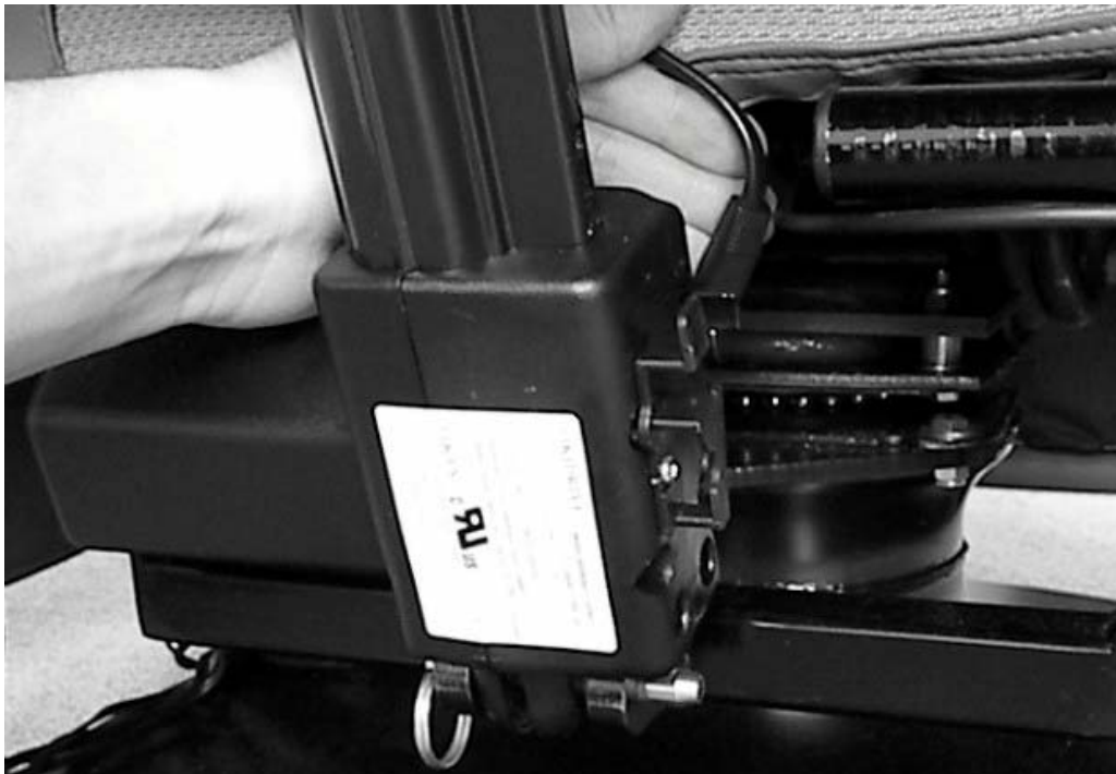
Figure 10 The recline power cable originating at the left rear of the seat frame connects to the power cable attached to the recline motor.
