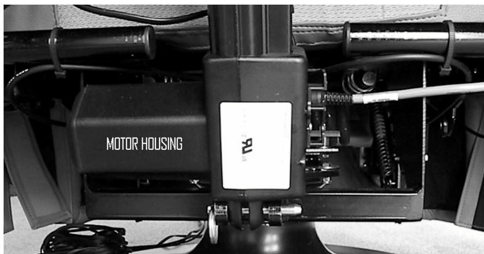
Figure 4 Detent pin extending through all of the holes in the bracket and bottom of the recline motor. Note recline motor housing facing to the left.
