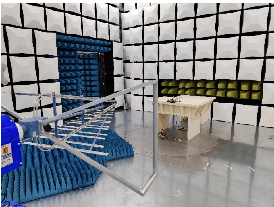
Photo No. 35: Test set-up 8.1, test antenna view
