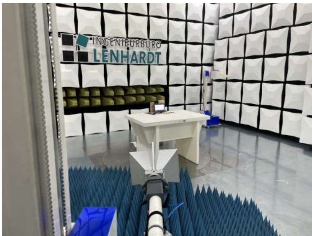
Photograph 32: Radiated emission 1...18 GHz
