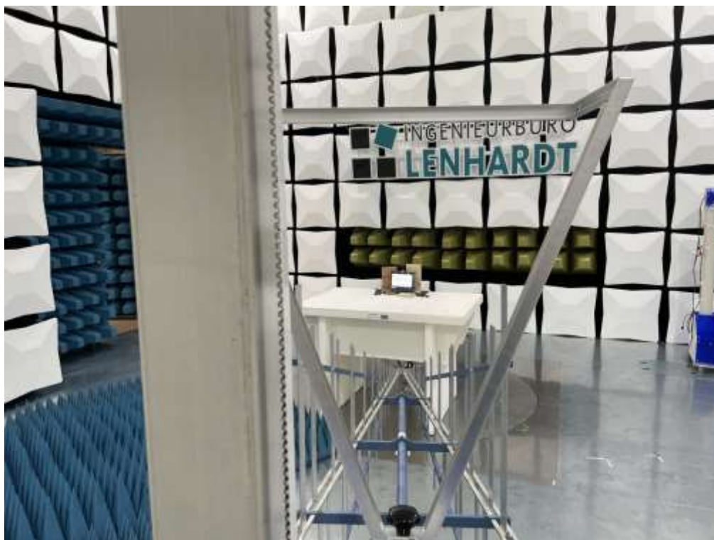
Photograph 31: Radiated emission 30...1000 MHz
