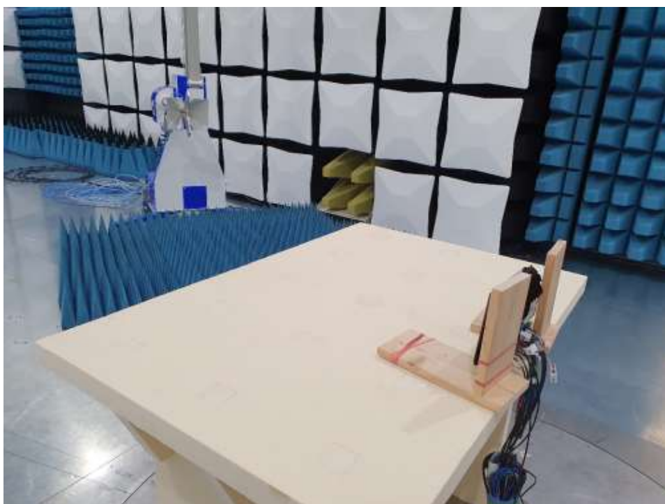
Photograph 8: Radiated emission 1...18 GHz
