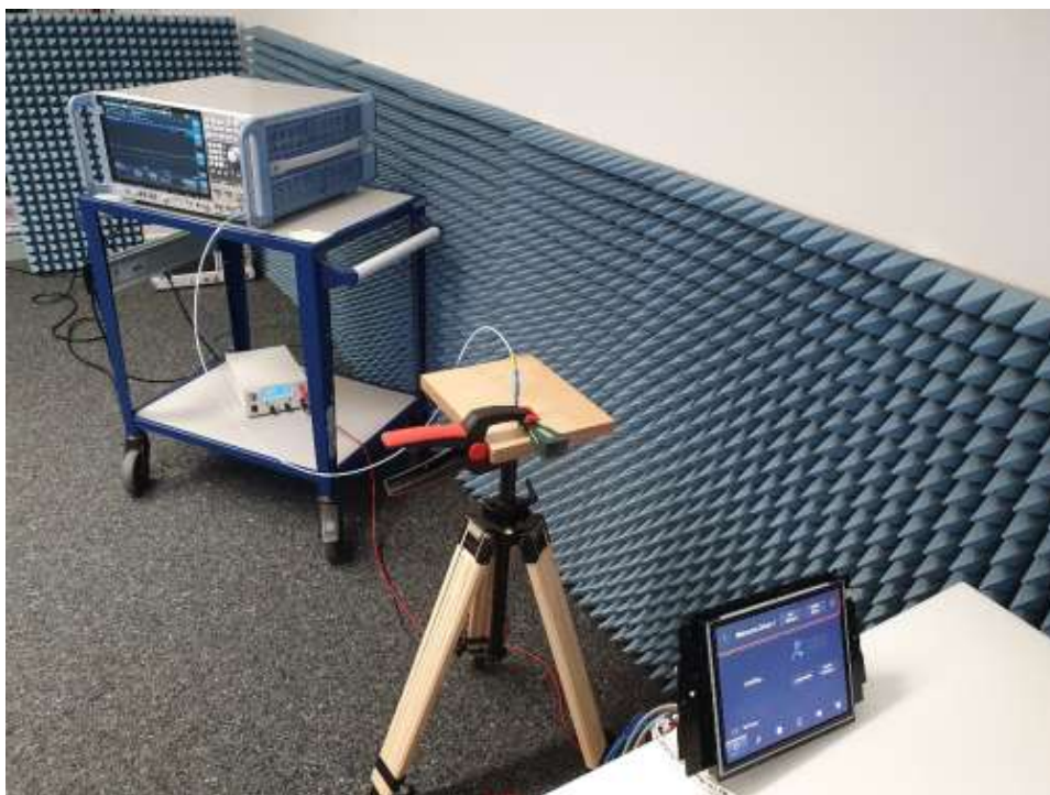
Photograph 3: Radiated emission 18...40 GHz
