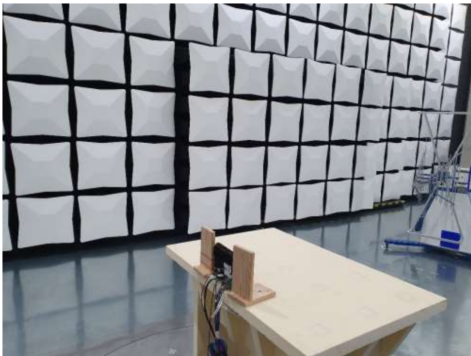
Photograph 4: Radiated emission 30...1000 MHz
