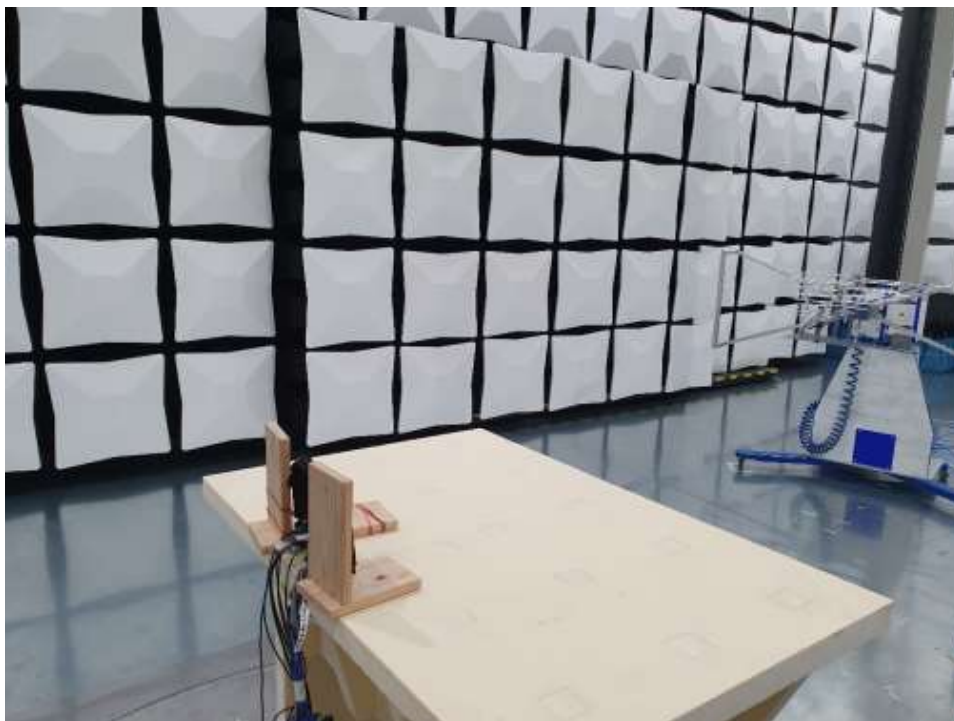
Photograph 7: Radiated emission 30...1000 MHz
