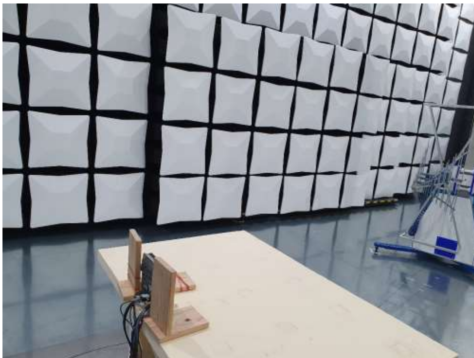
Photograph 22: Radiated emission 30...1000 MHz
