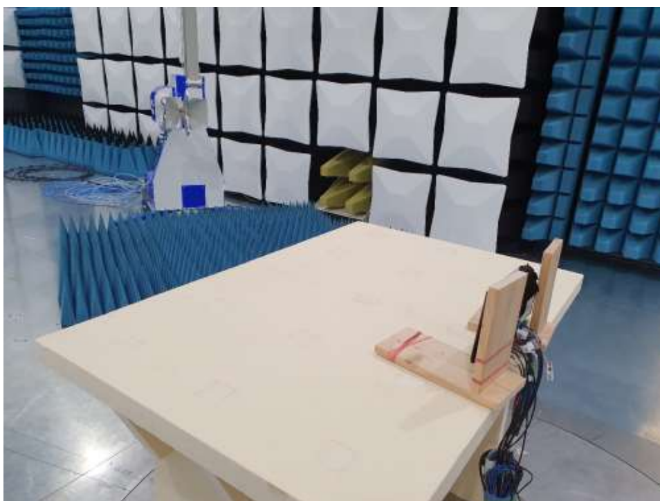
Photograph 5: Radiated emission 1...18 GHz
