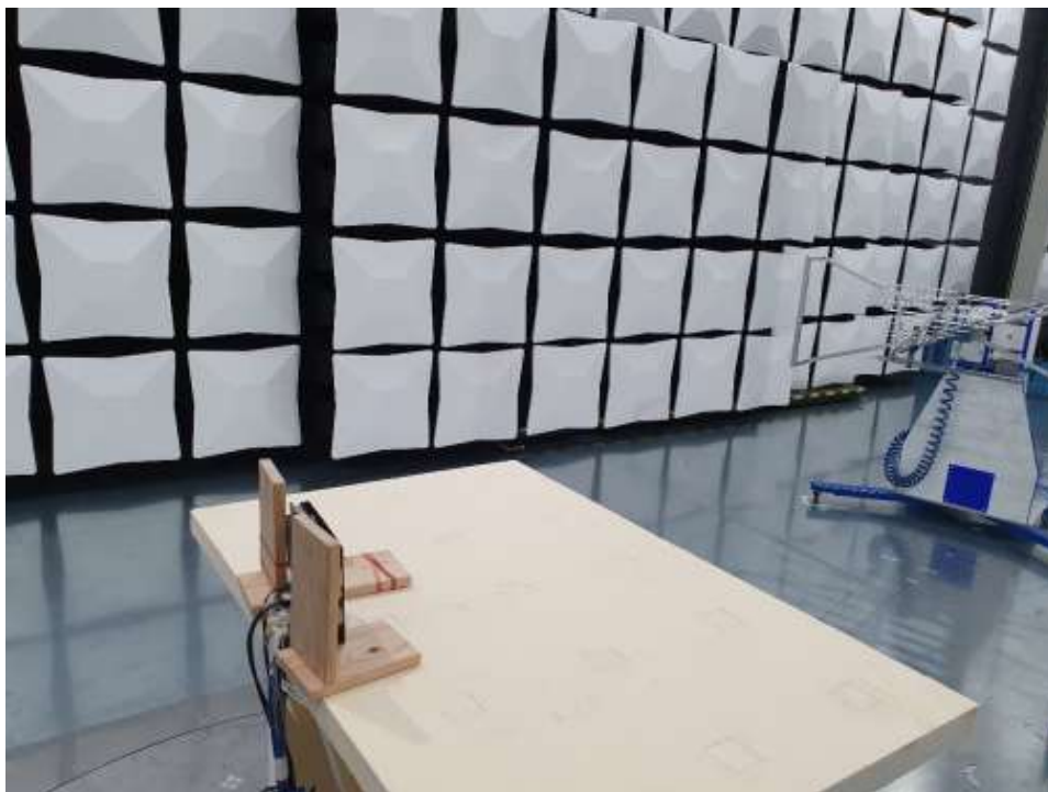
Photograph 10: Radiated emission 30...1000 MHz
