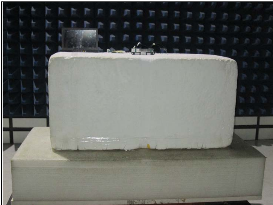
Radiated Emission Test above 1GHz
