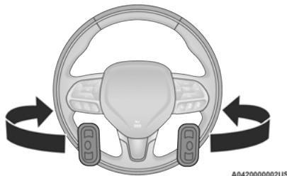
Remote Sound System Controls
