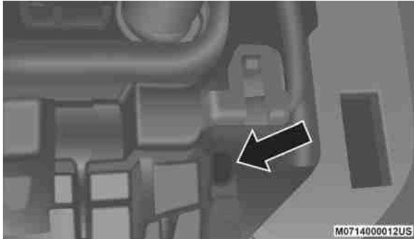
Gear Selector Override Location
