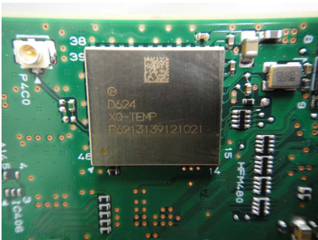
WLAN Module location
