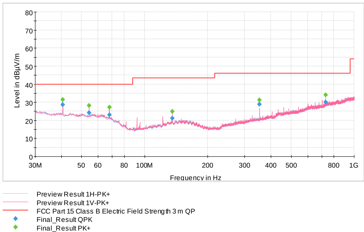
Figure 4. TX radiated emission 30 MHz to 1000 MHz, PCB antenna without TAG
