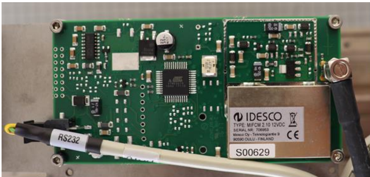
Photograph 4. The type label of the EUT2
