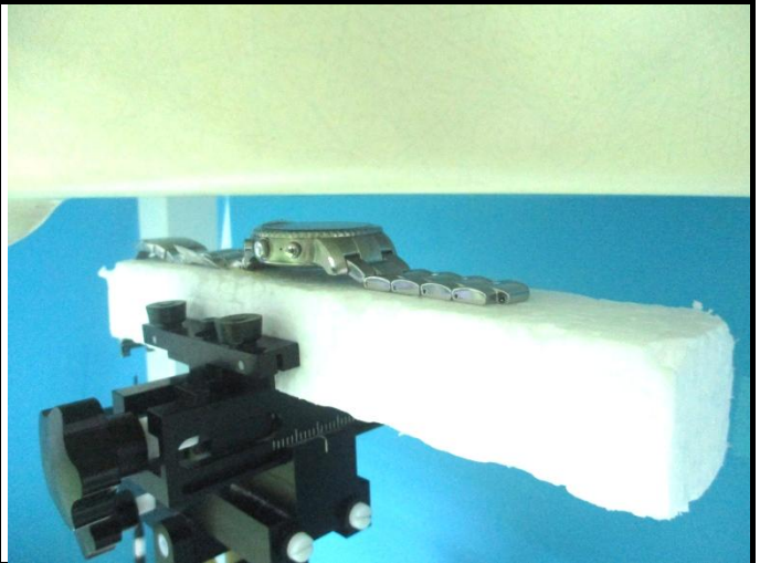
Front Face of EUT with 1 cm Gap for EUT 2
