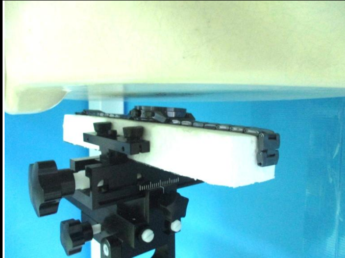
Front Face of EUT with 1 cm Gap for EUT 3
