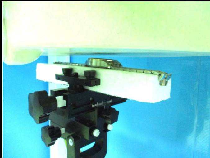
Front Face of EUT with 1 cm Gap for EUT 1
