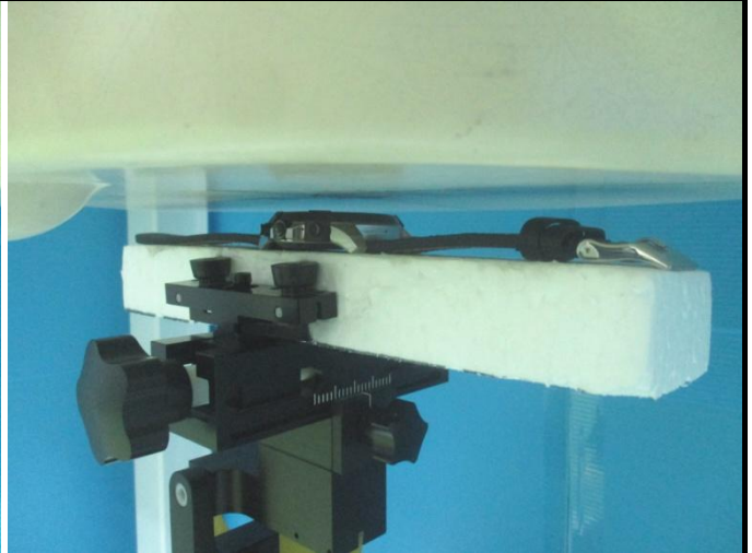
Front Face of EUT with 1 cm Gap for EUT 4
