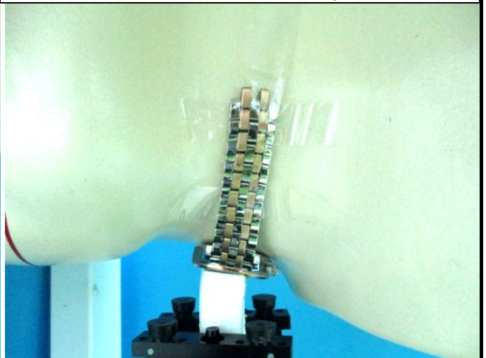
Rear Face of EUT with 0 cm Gap for EUT 1_Neck
