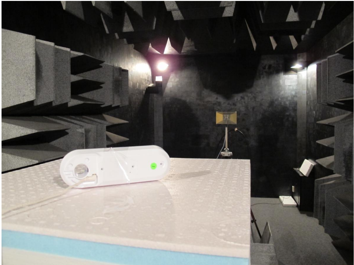
Photograph 1: Radiated emissions test set up, exploratory
