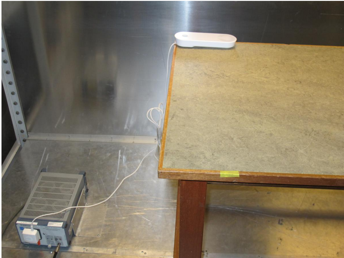
Photograph 4: Conducted emissions test set up
