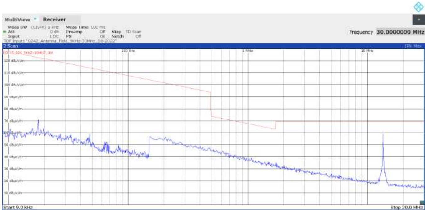
The highest peak is the RFID 13.56 MHz carrier frequency.
