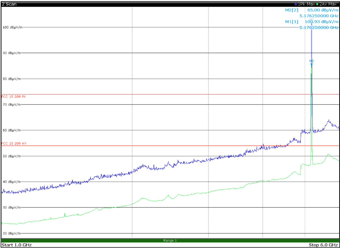
Figure 7.4-3: Radiated spurious emissions 1 to 6 GHz, 5180 MHz with antenna in vertical polarization
