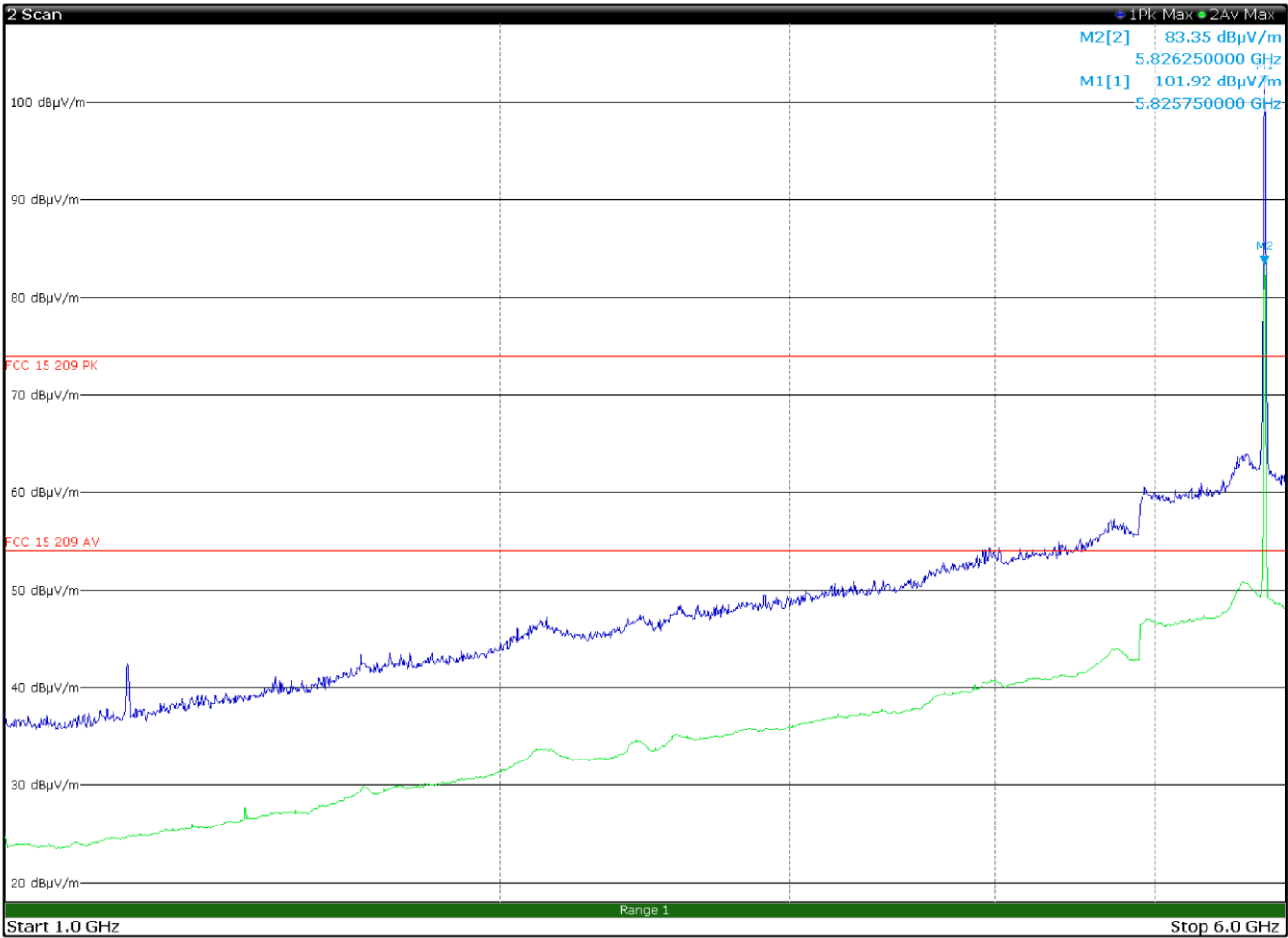
Figure 7.4-11: Radiated spurious emissions 1 to 6 GHz, 5825 MHz with antenna in vertical polarization Limit exceeded by the carrier
