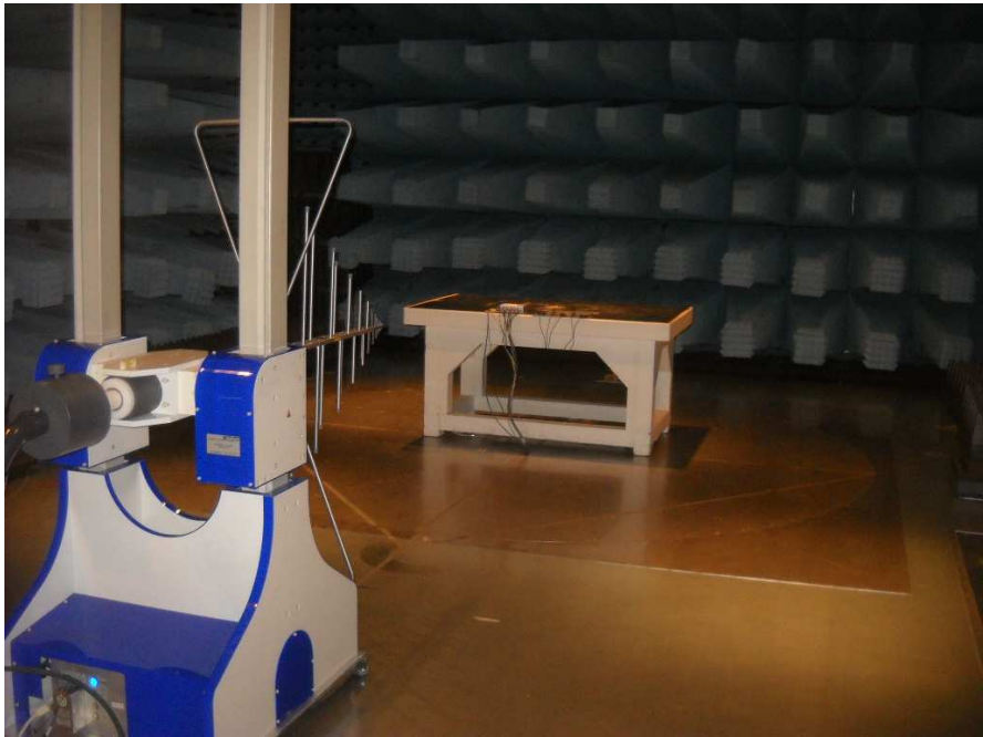
Radiated emission below 1 GHz with EUT in configuration 2
