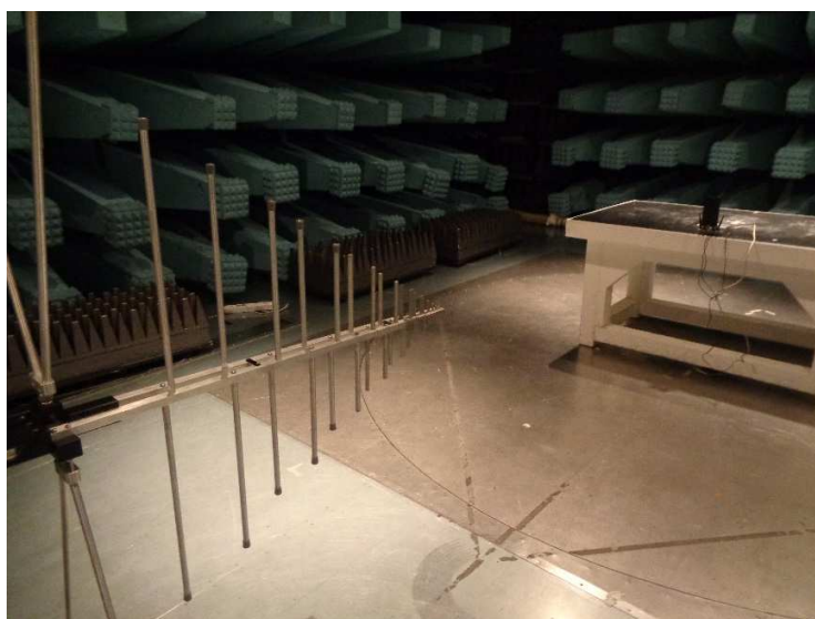
Radiated emission below 1 GHz – Antenna configuration 2
