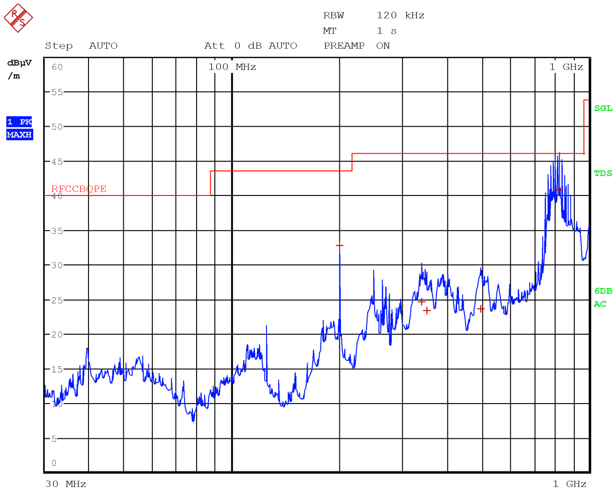
Figure 8.1-1: Radiated spurious emissions with WCDMA at 1880 MHz and WIFI at 2437 MHz – antenna in horizontal polarization
