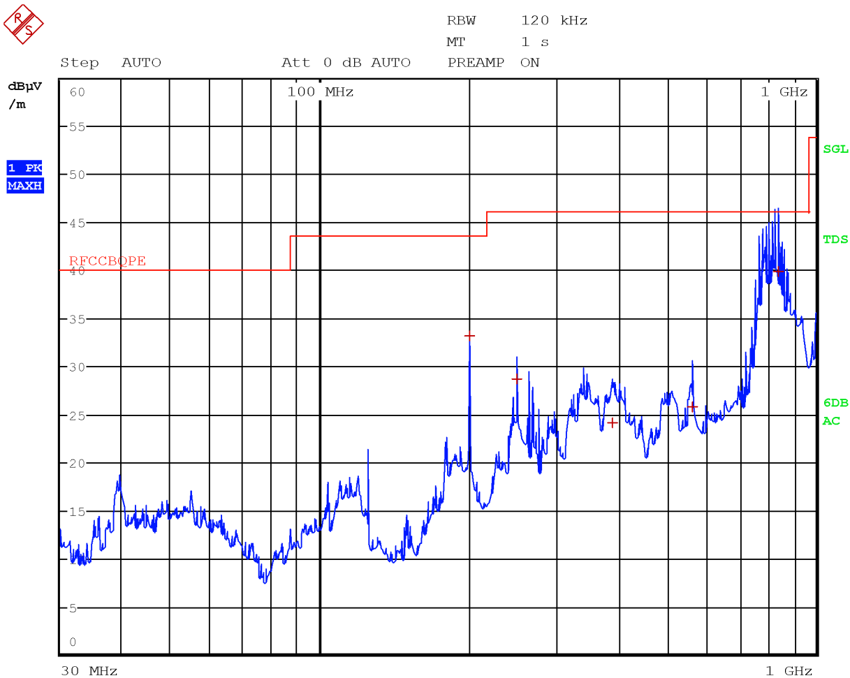
Figure 8.1-41: Radiated spurious emissions with WCDMA at 1732.6 MHz and WIFI at 5200 MHz – antenna in horizontal polarization
