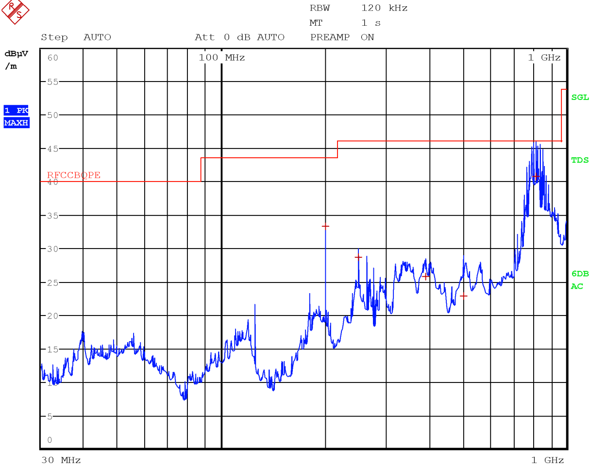
Figure 8.1-11: Radiated spurious emissions with WCDMA at 1732.6 MHz and WIFI at 2437 MHz – antenna in horizontal polarization
