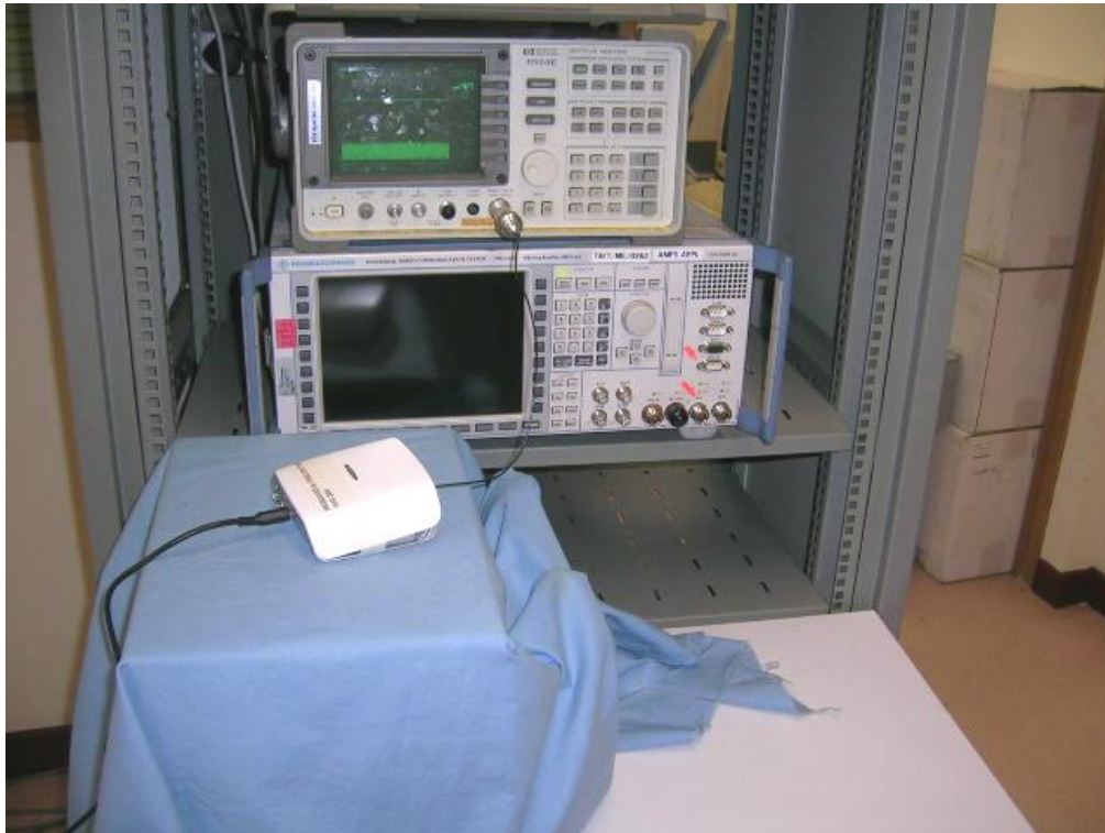
Average Frequency Dwell Time Test Setup
