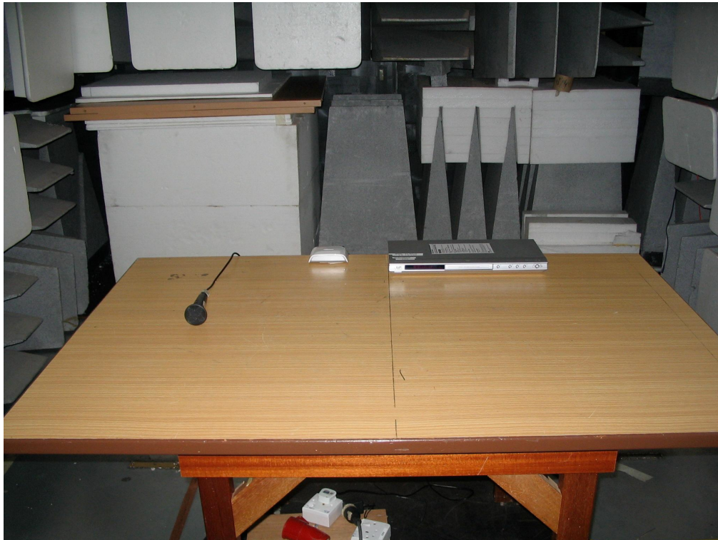
Radiated Emissions Test Setup (Front View) - Transmitter
