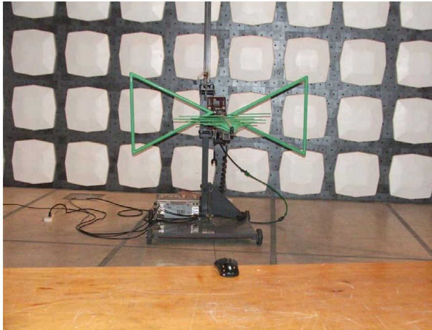
Radiated Emissions Test Set-up (Low frequency)
