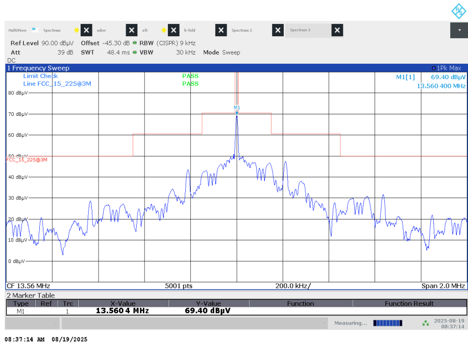
Plot 3: Spectrum mask (the limits are recalculated according to the ANSI C63.10-2020 sub clause 6.4)
