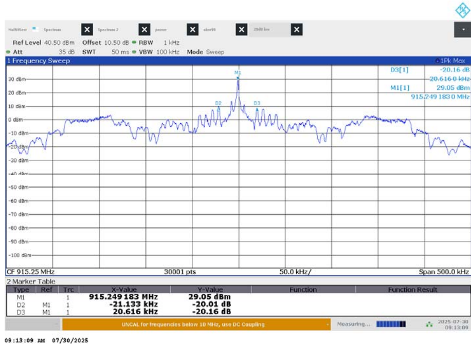
Plot 3: tx 915.25 MHz – 20 dB bandwidth
