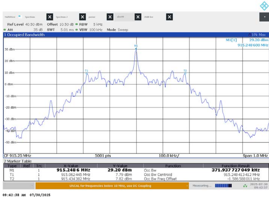
Plot 4: tx 915.25 MHz – 99% bandwidth
