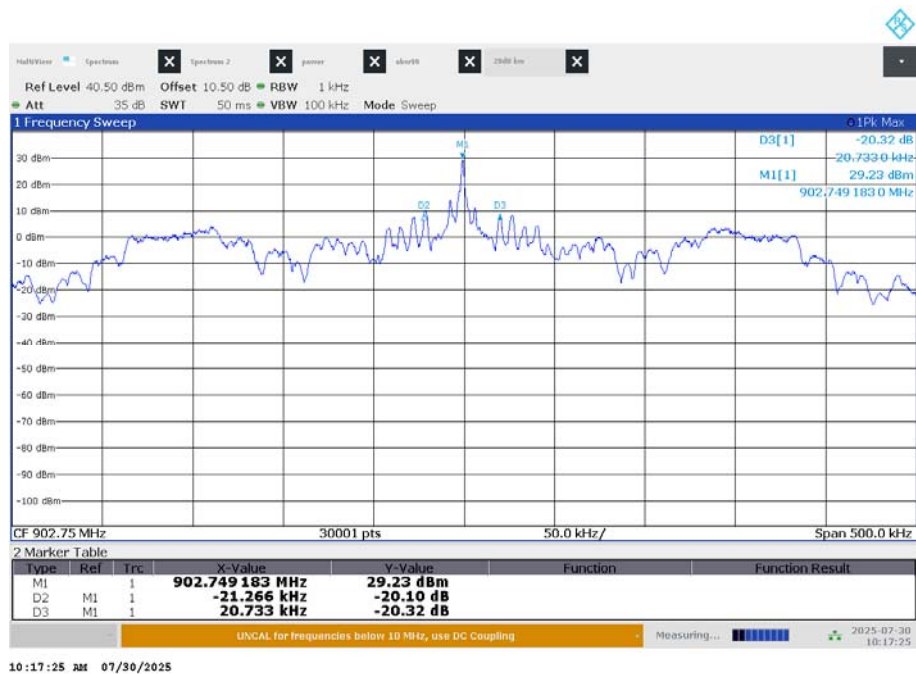
Plot 1: tx 902.75 MHz – 20 dB bandwidth
