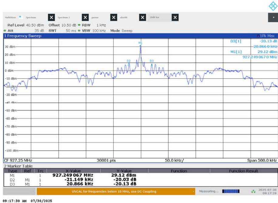
Plot 5: tx 927.25 MHz – 20 dB bandwidth
