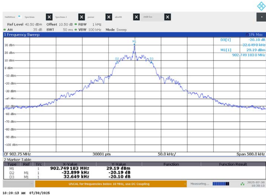
Plot 1: tx 902.75 MHz – 20 dB bandwidth
