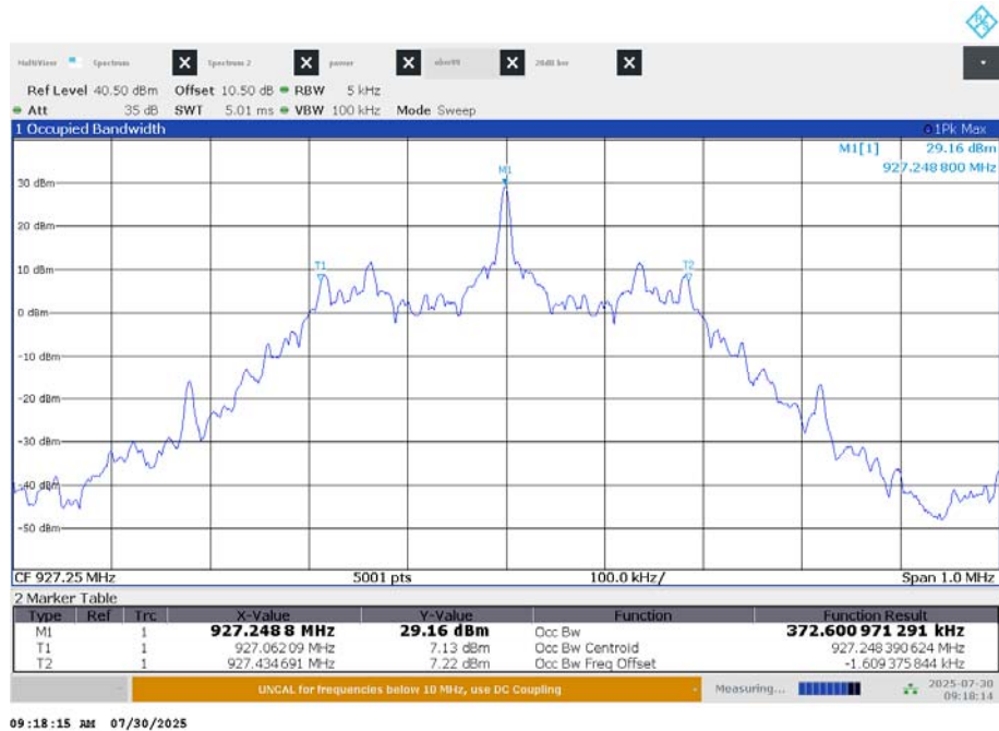
Plot 6: tx 927.25 MHz – 99% bandwidth
