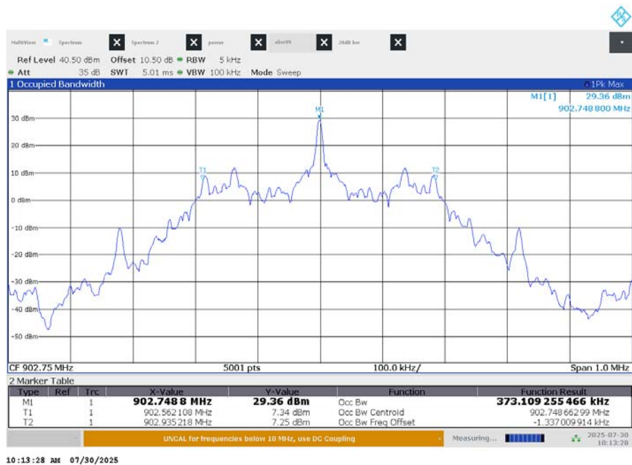
Plot 2: tx 902.75 MHz – 99% bandwidth
