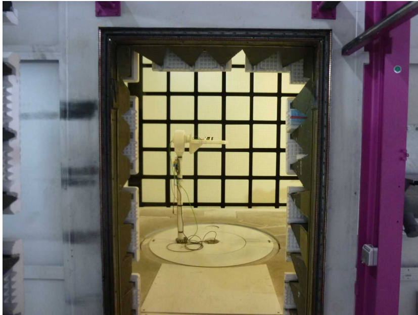
Photo 1: EUT at the anechoic chamber, test setup without tag
