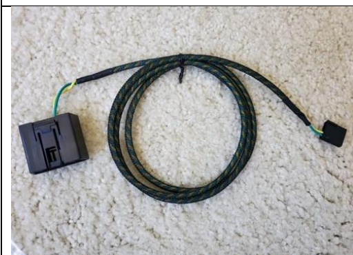
OBD-II Data Only Cable Only included in kits for OBD-II networks
