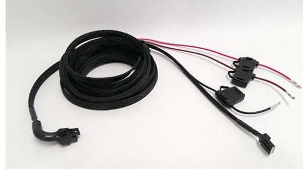
Non-ECM, Device Power Only Cable with inline fuses: Red and Black wires = 5-amp fuses Brown wire = 1-amp fuse
