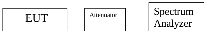
Block Diagram 2. Power Output Test Setup
