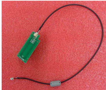
Antenna with cable
