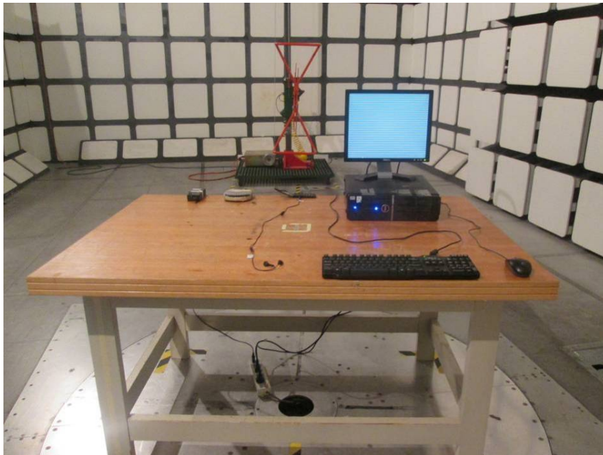
Radiated Emissions – Front View (Below 1 GHz)
