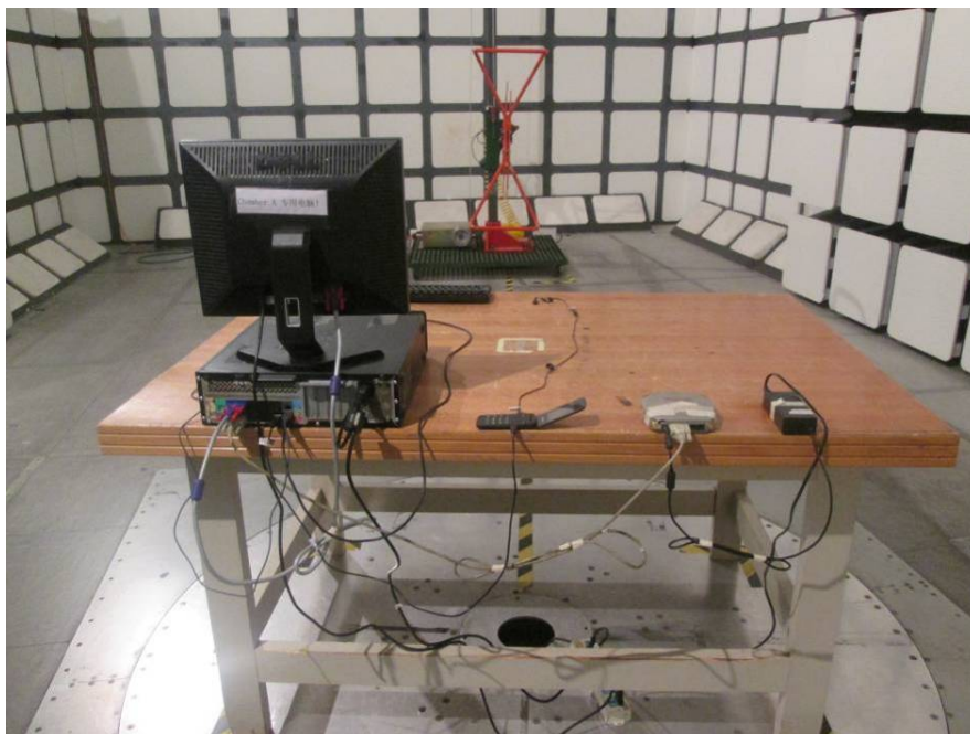
Radiated Emissions – Rear View (Below 1 GHz)
